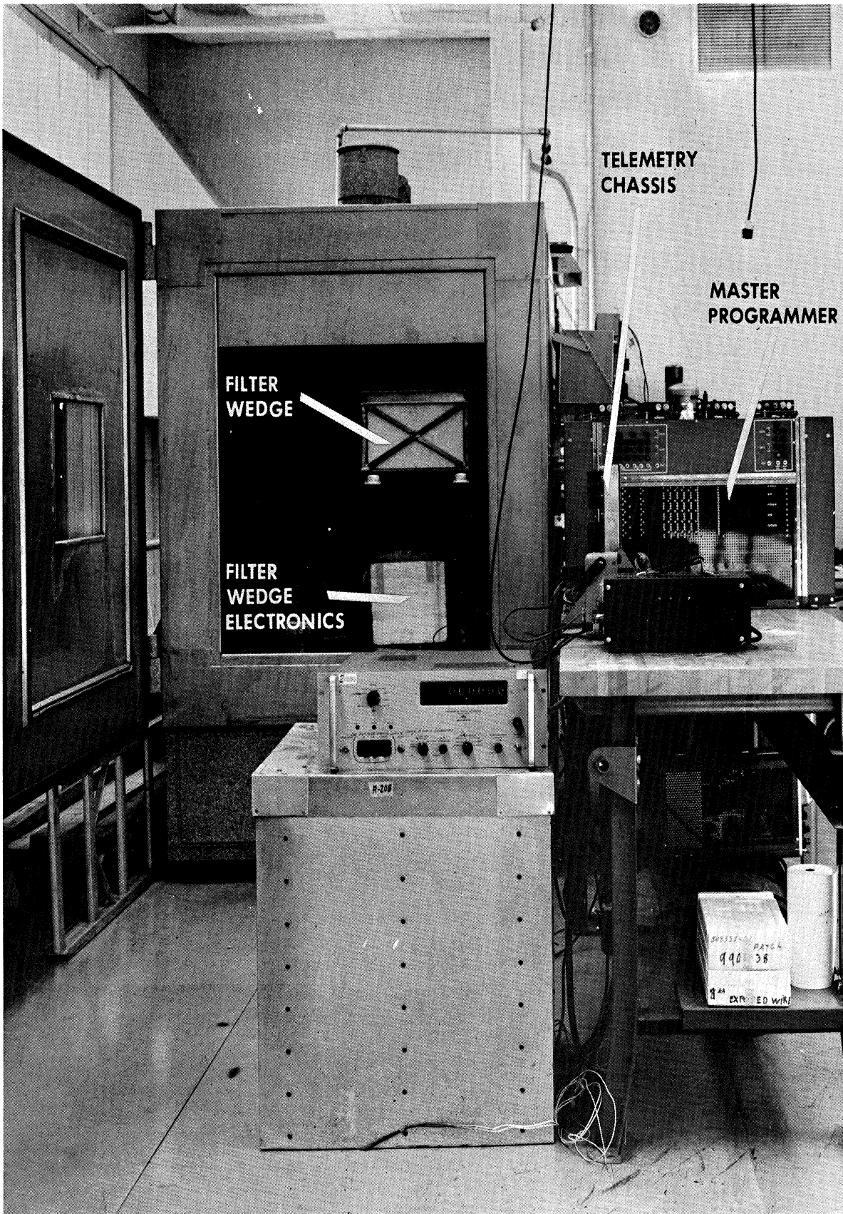
Fig. 2 Filter-Wedge test configuration, instrument in test chamber
