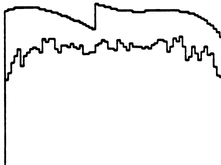
Figure 5.1. An Anomalous Break in Parameter Curve for Noisy Torus
