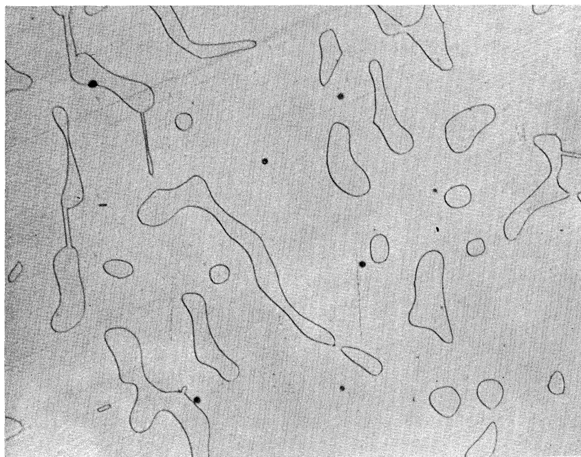
U of M No. R-1 CF8M Stainless Solution Quenched R-2 from 2050°F X500 Electrolytic R-3 Etch
