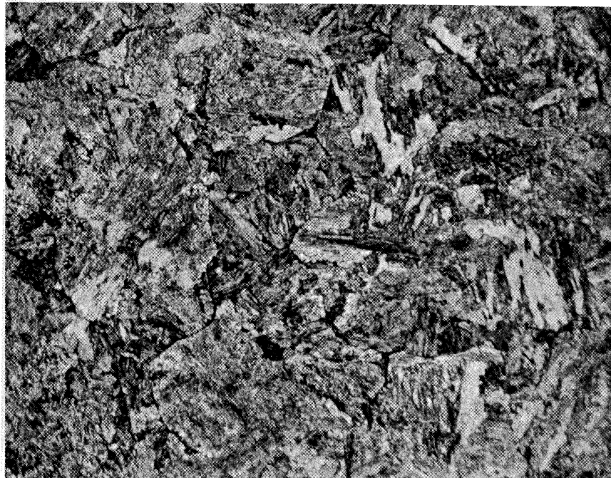
U of M No. H-1 45A7 (Carbon Chrome Moly Steel) H-2 Normalized and Tempered H-3 X500 2% Nital Etch
