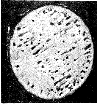
N-2 Arcos Stainlend WLR 16.36 mg/hr 7 hr. exposure
