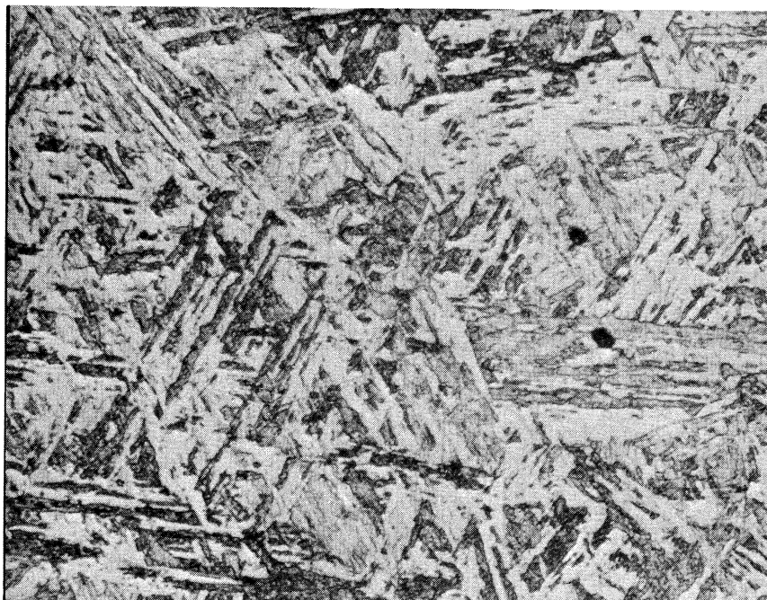
U of M No. J-1 CA15 - Low Cr, Low Si, structure containing no Ferrite. Normal properties J-2 J-3 X500 Ferric Chloride Etch
