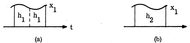
FIGURE 30. THE MEASUREMENT OF x_1 . (a) Two steps each of interval length h_1 . (b) A single step of interval length h_2 = 2h_1 .
