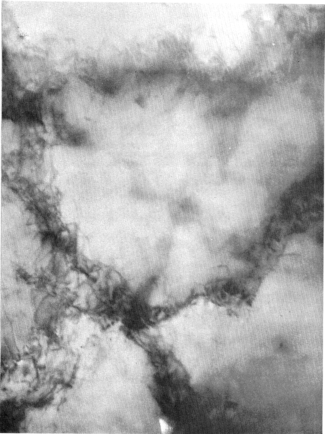
Figure 4.4. Sub-grain boundaries in an 80% cold rolled, recovered specimen which was strained an additional 0.2% after recovery. 20,000x.
