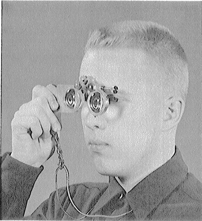
FIG. 9 HAND-HELD MOUNT FOR THE NIGHT TELESPECTACLE ELEMENTS
