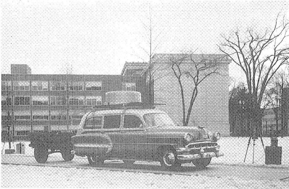
FIG. 4 STATION WAGON INSTALLATION OF RECORDING POLAR NEPHELOMETER
