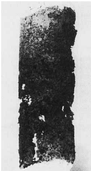
Figure 8. Wood's alloy casting of coreflood run in dolomite at a high injection rate.
