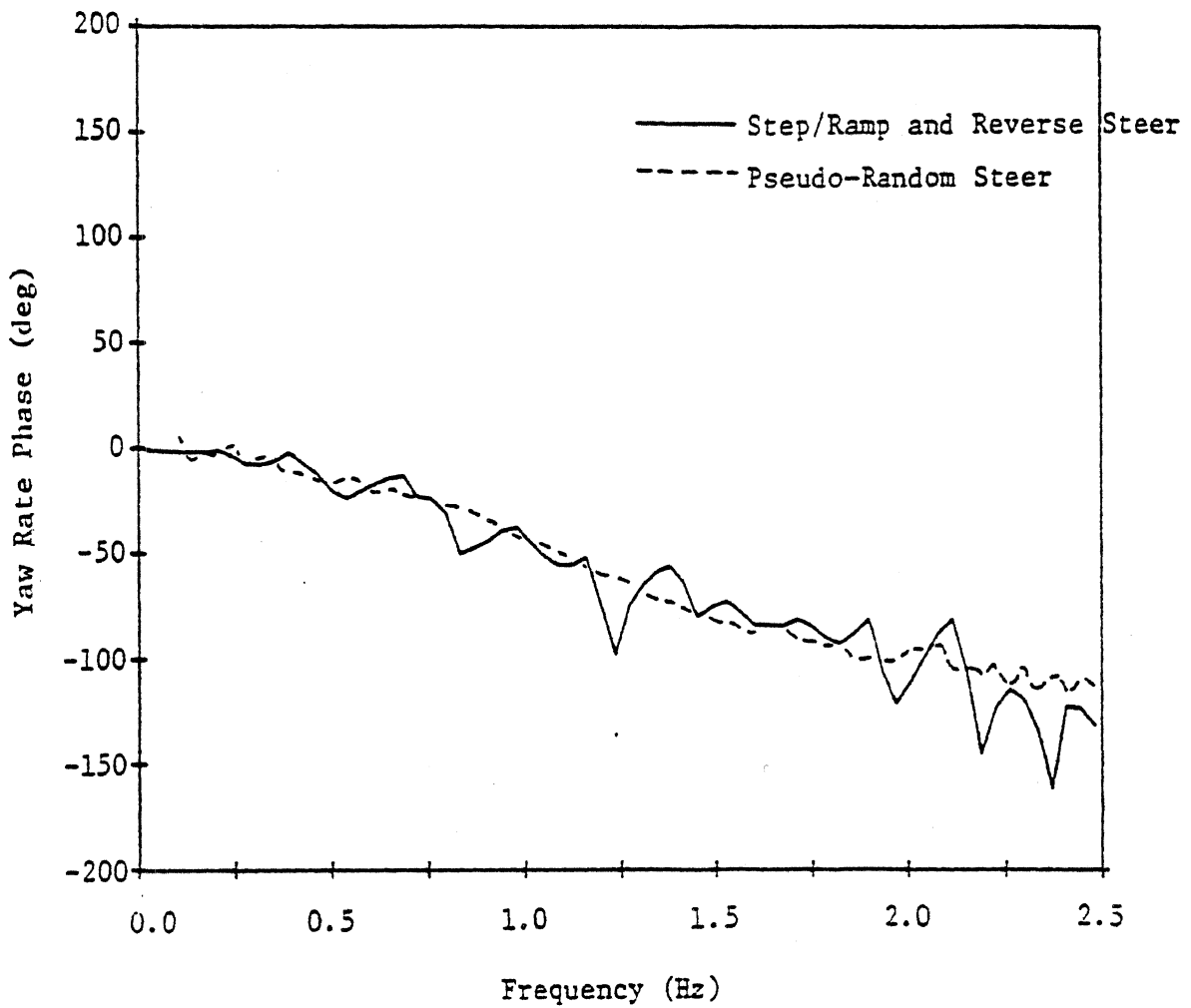
Figure 20b. Transfer functions from pseudo-random and step/ramp-reverse steer inputs, yaw rate phase
