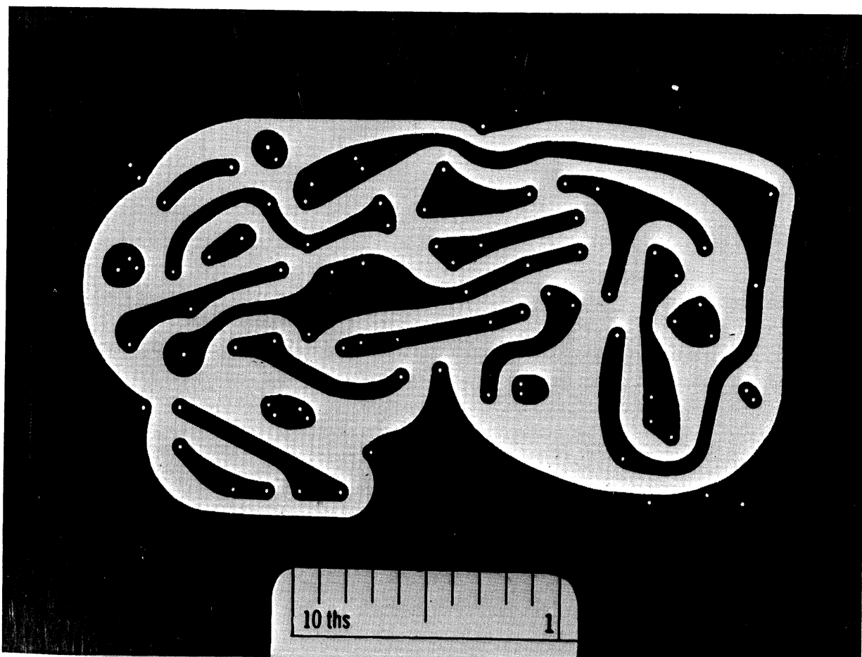
Fig. 59. Wiring Connections on Printed Circuit Board.
