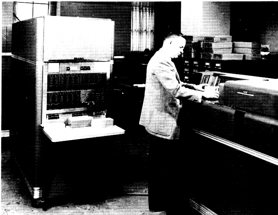
Figure 10. Console and "Read-Punch" Unit of The University of Michigan IBM 650 Digital Computer.
