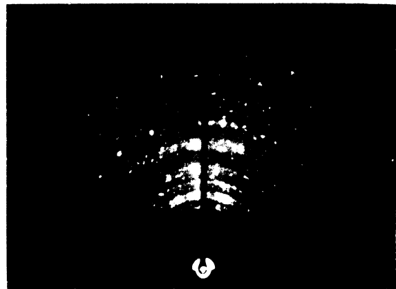
d. Pattern of Cb(C-N) and Possibly M_{23}C_6 from N-155 Alloy.
