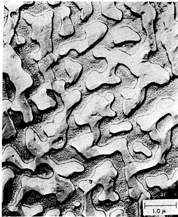
Fig. 8. Replica of Cu film on NaCl after heating to 630°C for 10 min.
