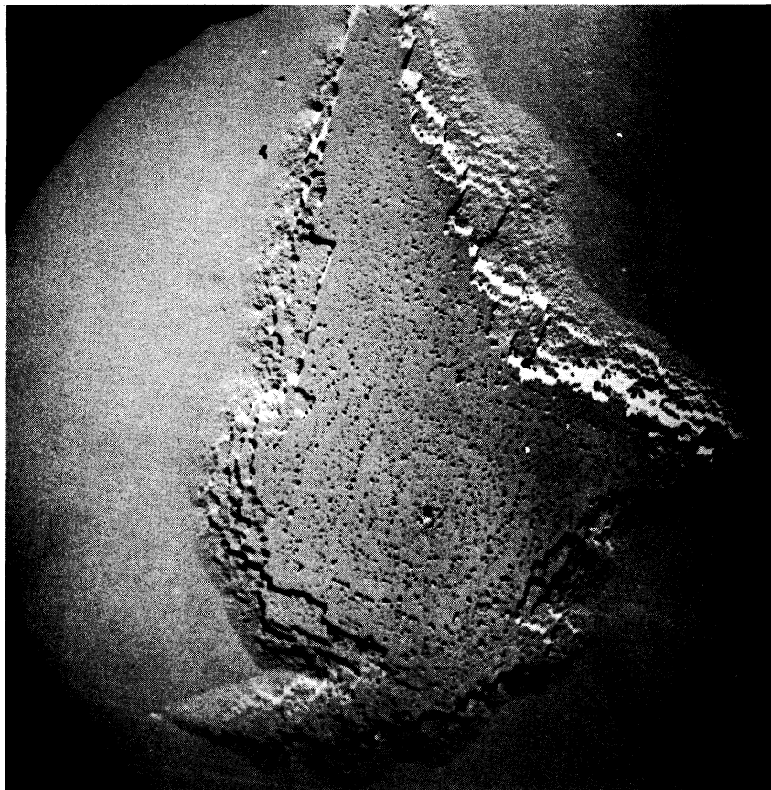
Fig. 22. Replica of Cu film on KCl after heating to 630°C for 10 min. (3000x magnification).
