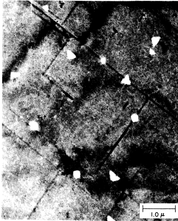
Fig. 26. Micrograph of oxidized Cu film treated with HCl solution, 3 min oxidation.
