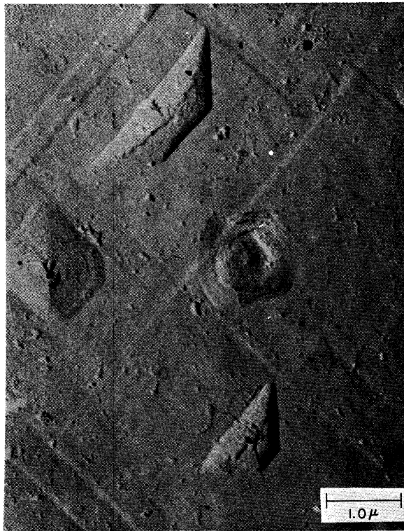
Fig. 25. Replica of substrate-annealed Cu oxidized in O_2 , 0.9 \times 10^{-3} torr, 525^\circ C , 15 min.
