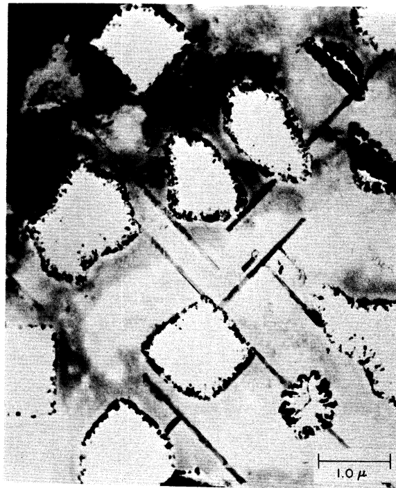
Fig. 29. Micrograph of oxidized Cu film treated with HCl solution, 15 min oxidation.
