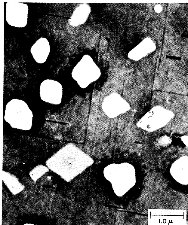
Fig. 27. Micrograph of oxidized Cu film treated with HCl solution, 5 min oxidation.
