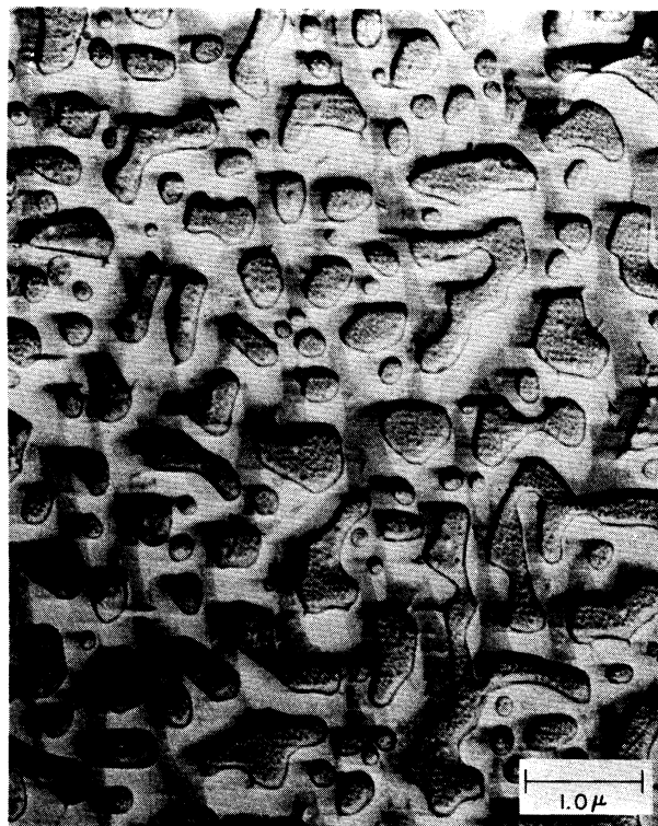
Fig. 9. Replica of Cu film on NaCl after heating to 630°C for 10 min.
