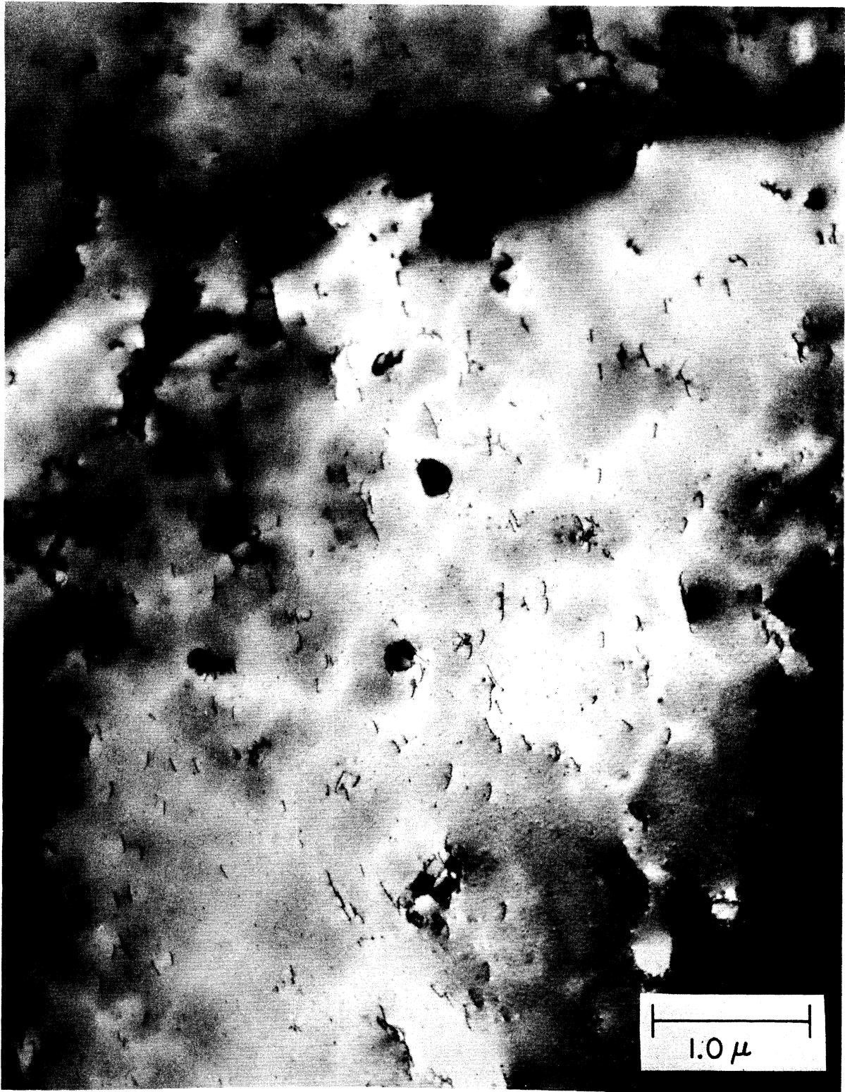
Fig. 16. Micrograph of Cu film heated to 630°C for 10 min after mounting on grid.
