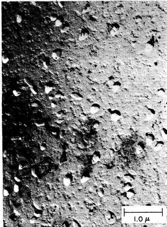
Fig. 36. Replica of Cu + 0.44% Te oxidized for 20 min.
