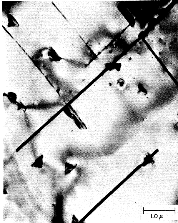
Fig. 24. Micrograph of substrate-annealed Cu oxidized in O_2 , 0.9 \times 10^{-3} torr, 525^\circ C , 2 min.
