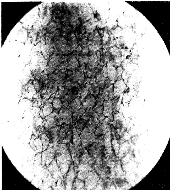
Figure 8. Cossettes Exploded from 60 psig to 22-inch Hg Vacuum (10 minutes)
