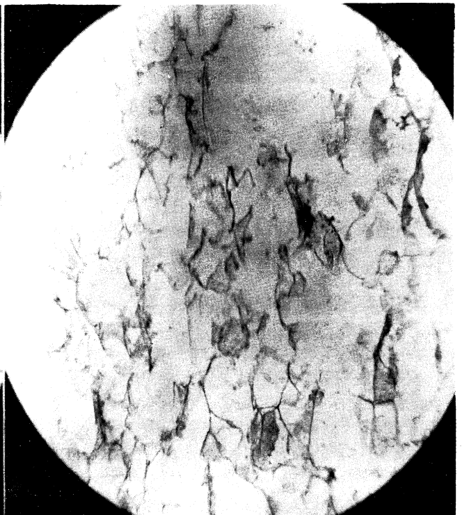
Figure 13. Cossettes Exploded from 110 psig to 22-inch Hg Vacuum (7 minutes)
