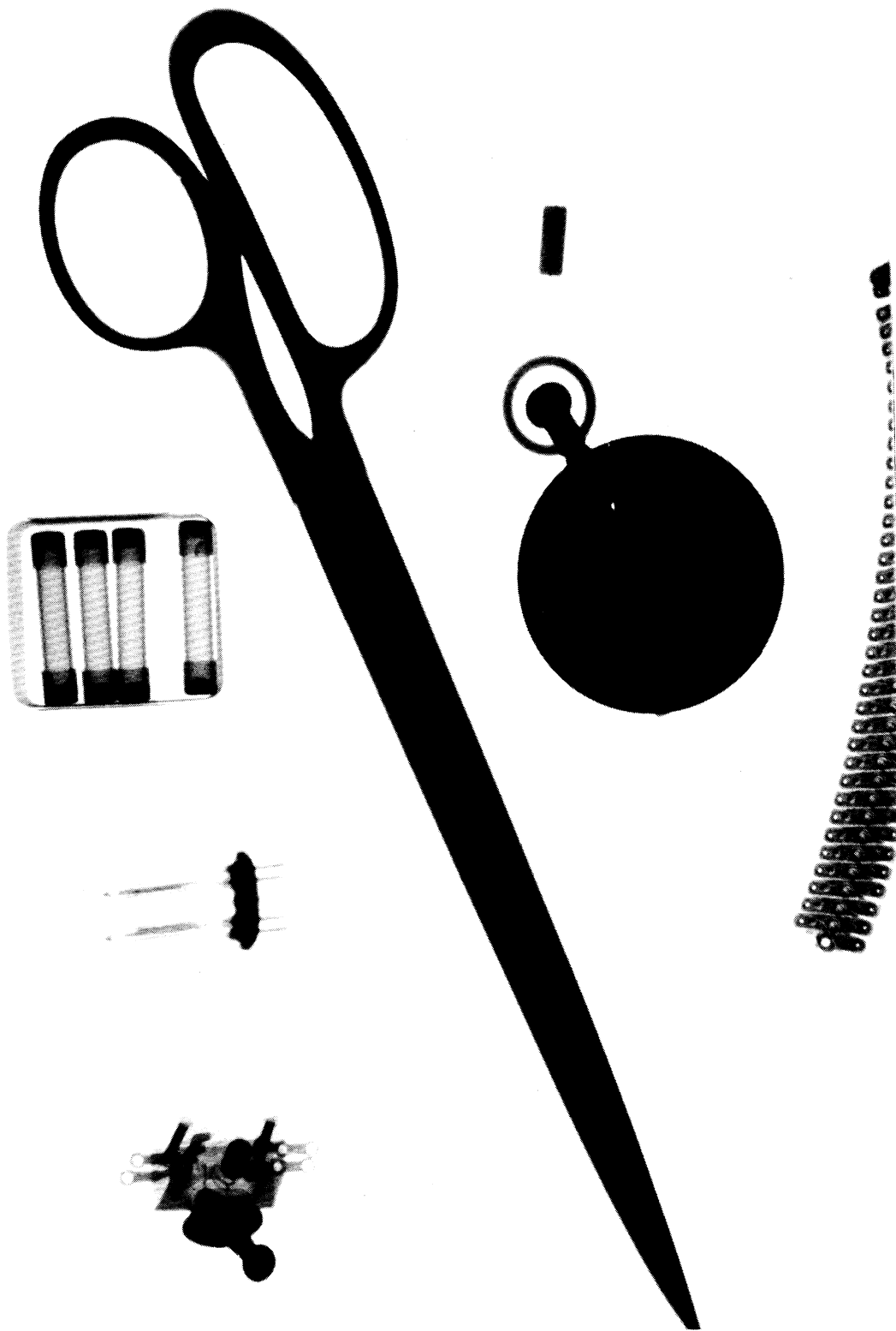
Fig. 6. Technical radiograph with promethium-147 tungstate source; 1-curie Pm, 44 hr at 10 in.
