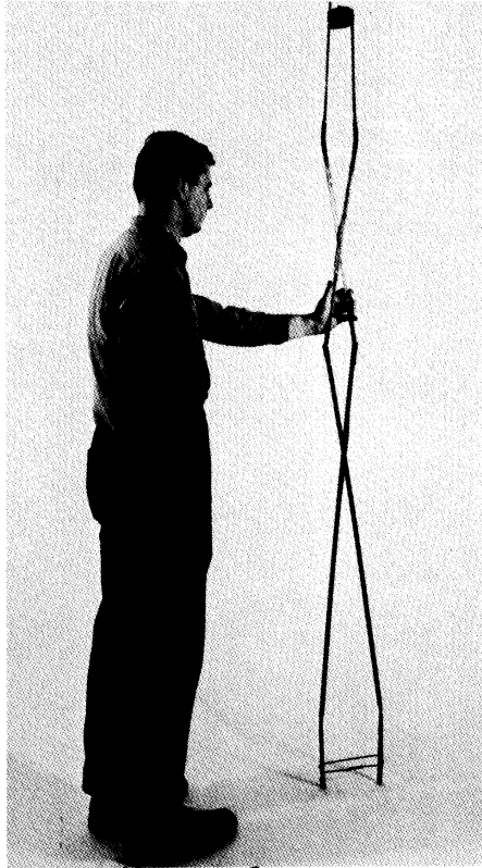
Willow Run Fig. 12. Special Tongs for Fastening and Removing Head of Burner.
