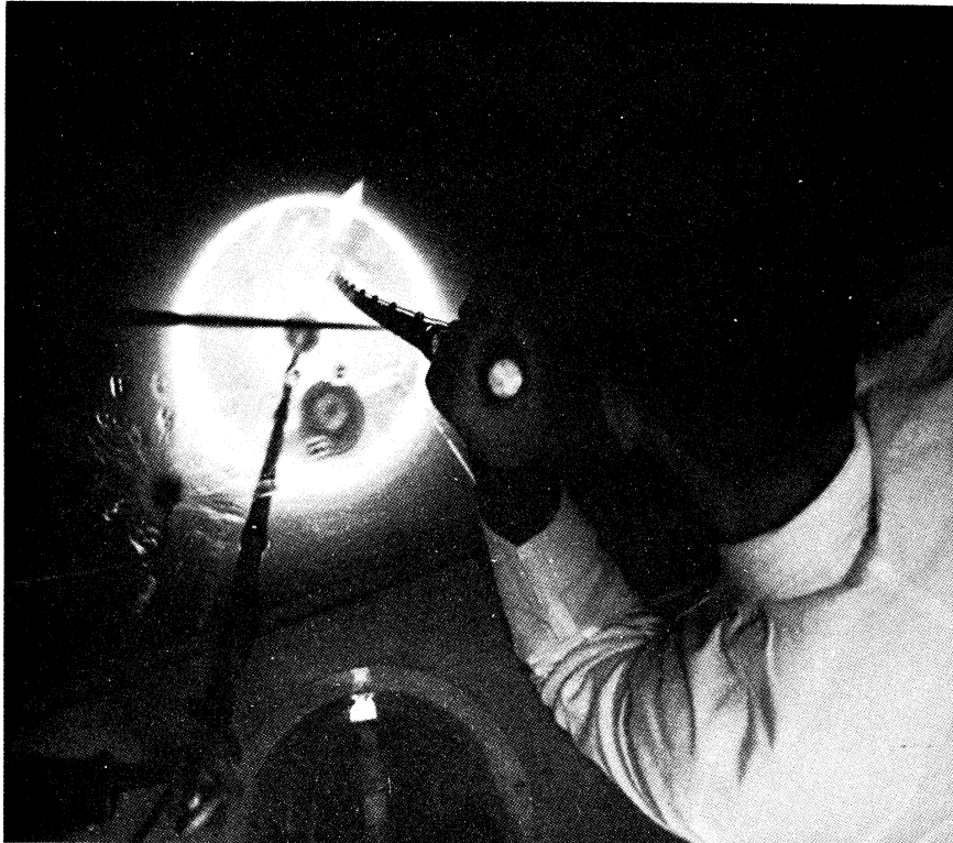
Fig. 94a. Loading Cobalt Rods Into Holder in 14 Feet of Water Using Submarine Light and 18 Foot Tongs.
