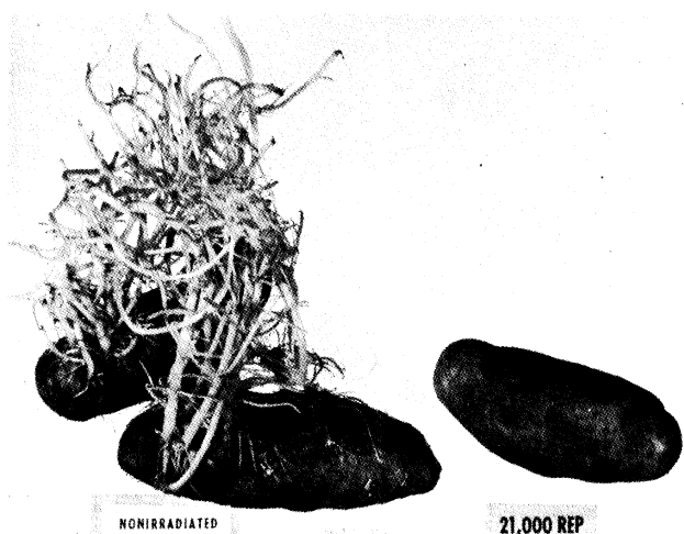
Fig. 35. Idaho-Grown, Burbank Russet Potatoes of the 1953 Crop. Irradiation Performed May, 1954. Stored at 50°F until Photographing September, 1954.
