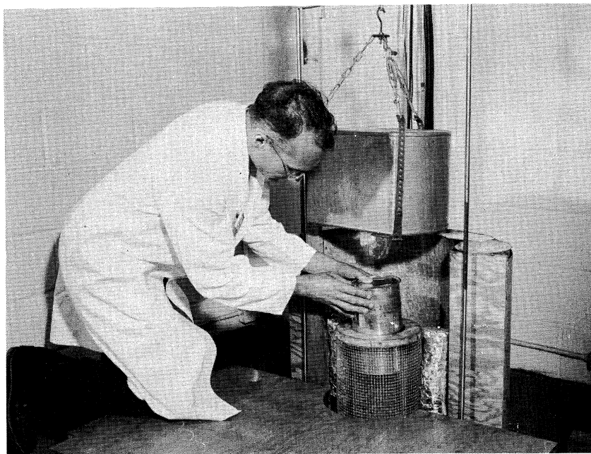
Fig. 3. View of the three containers used for the irradiation of wet mash.
