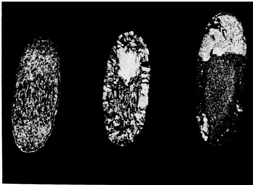
Fig. 27. Three Successive Primary Turns of A Filament after Showing Cold-worked, Fine-grained, and Coarse-grained Structures. (250X)
