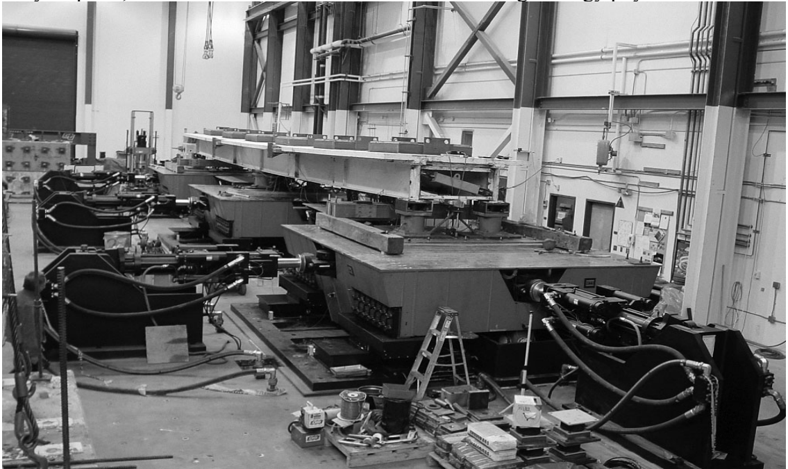
Figure 2 Reduced scale bridge deck positioned on 3 biaxial shaking tables (Image courtesy of the University of Nevada)
