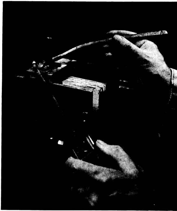
Photograph 16. Welding the Cell Post to the Cell Plate Strap.
