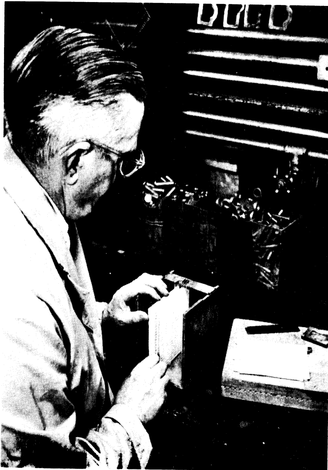
Photograph 13. Assembly of Plates in Burning Comb.
