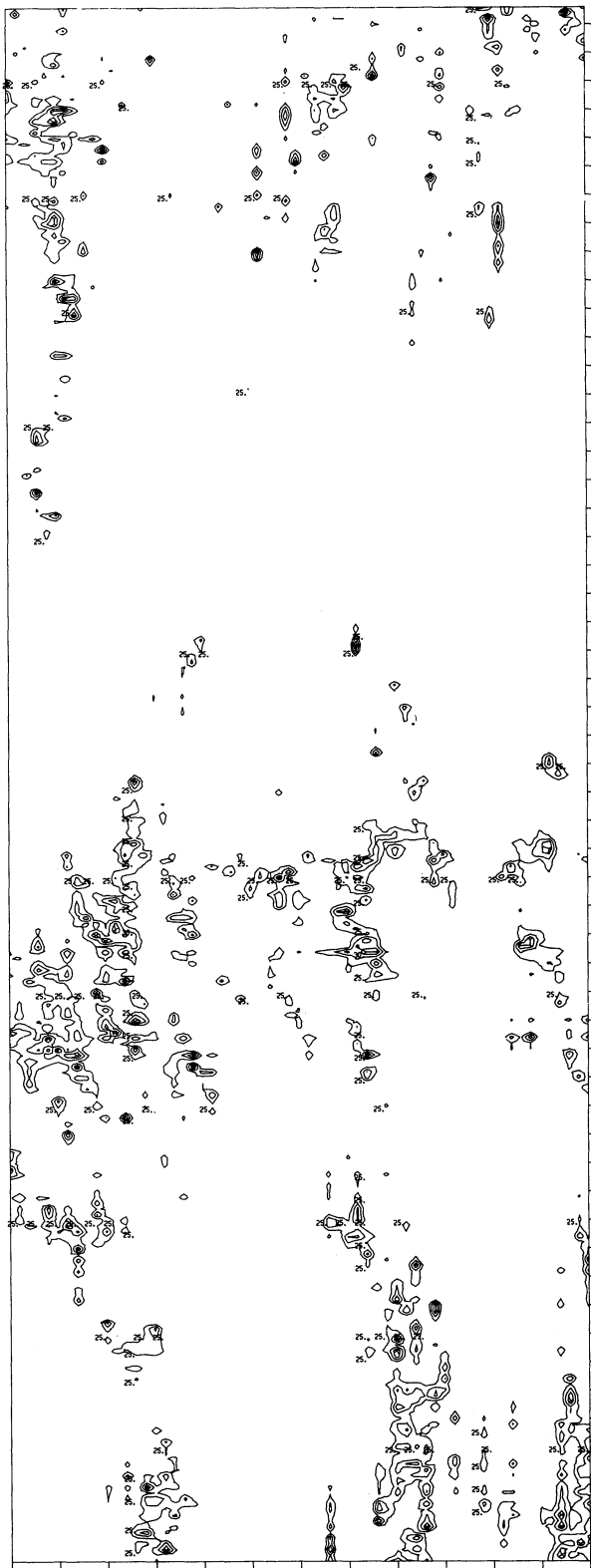
Fig. 5.5. Contours of the relative path loss function at 25, 30, and 35 dB relative path loss. The 25 dB contour is at the estimated wide-band noise level
