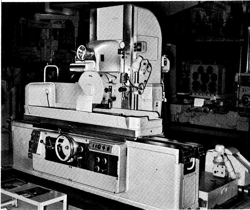
Fig. 14. Surface Grinder produced by Moscow Grinding Machine Works, Table size 15 x 75 inches.
