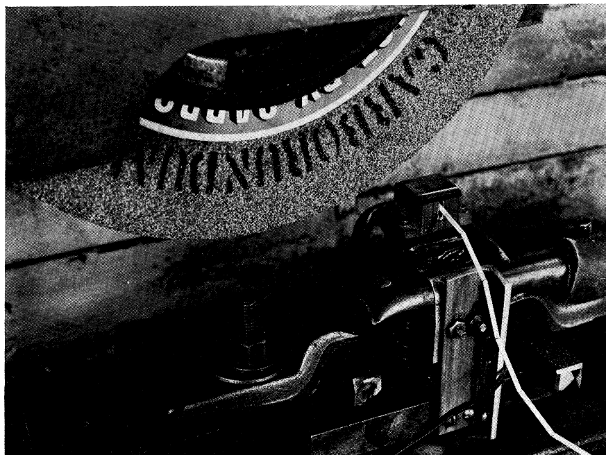
Fig. 22. Close-up view of the grinding specimen mounted on top of the magnetostrictive transducer clamped at nodal points to the table of the surface grinder. The thermocouple imbedded in the underside of the work specimen is led out through the ceramic insulators shown at the right. Work piece oscillates alternately from right to left underneath the grinding wheel.
