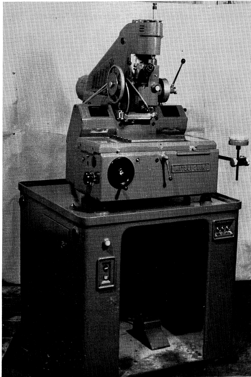
Fig. 9. High Precision Jig Borer, No. 0, by Mitsui Precision Machinery and Engineering Company, Ltd.
