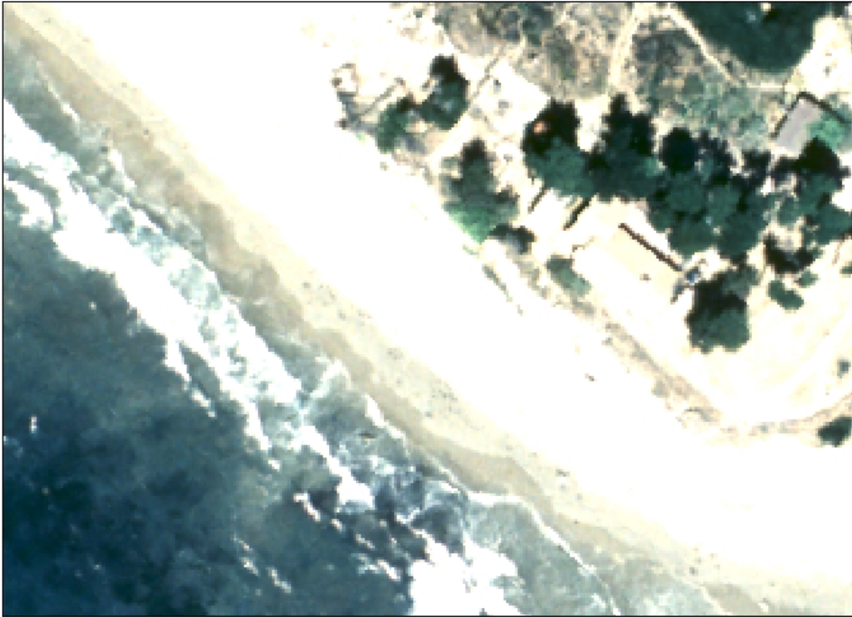
Figure 5: High water line is visible in the above image (a portion of the georeferenced 2001 photo) as the change in color from the bright white sand to the yellow colored sand. The grey sand shows the current wave swash area. By adjusting the brightness and contrast of the images, these features can be clarified.
