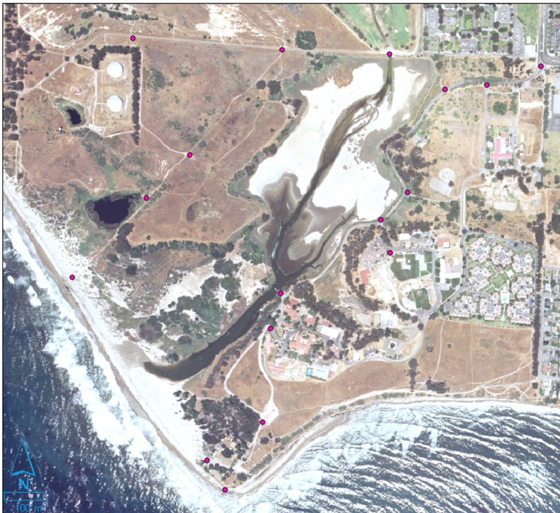
Figure 4: Location of ground control points shown on a georeferenced photo from 1997.
