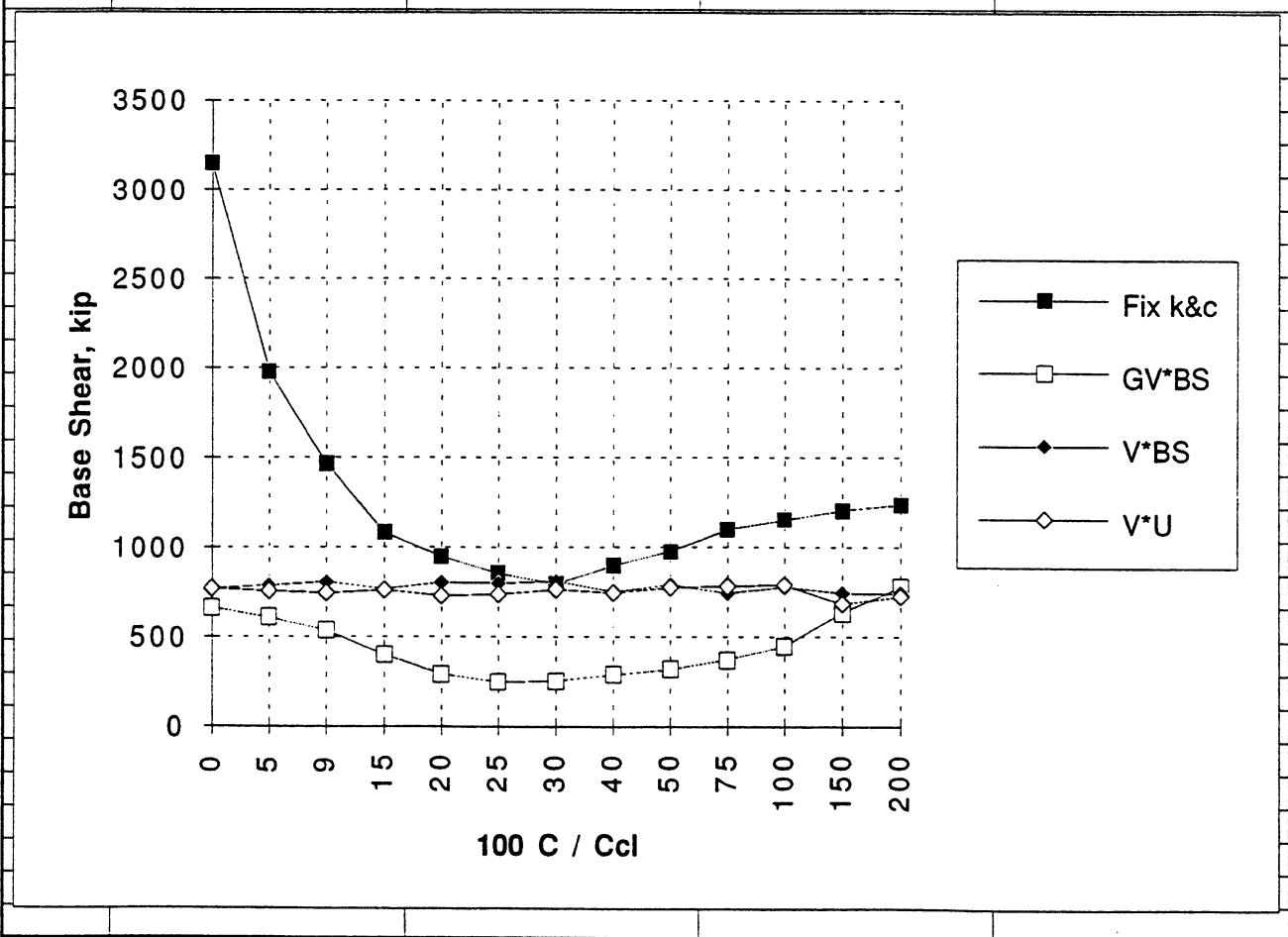
Section I, System B, Case 3, Base Shear
