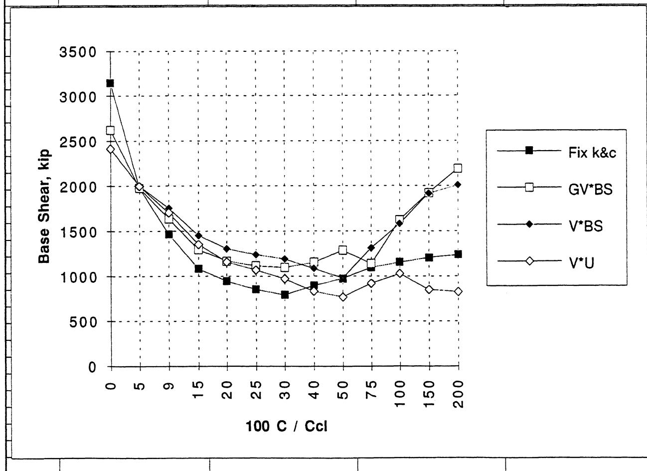
Section I, System C, Case 3, Base Shear
