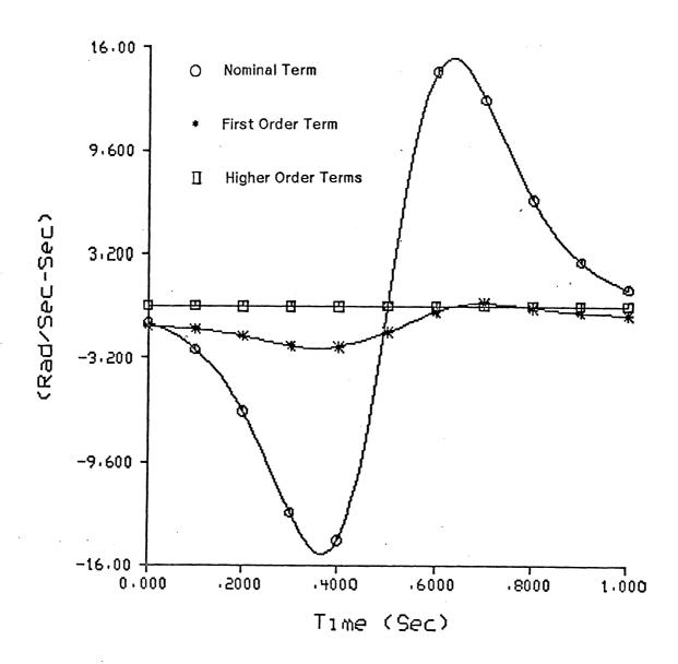
Figure 4 Contributions of the First Order Term and the Higher Order Terms in the Linearization of the Dynamic Model ( Joint 2 )
