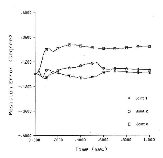
Figure 10 Adaptive Controller: Case (b)
