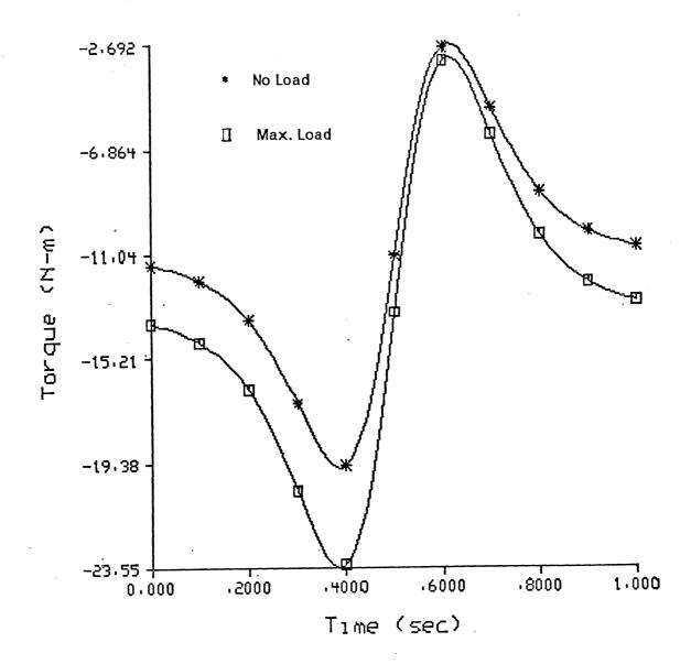
Figure 14 Variation of the Applied Torque ( Joint 3 )
