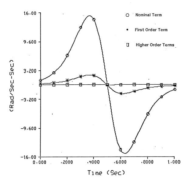
Figure 3 Contributions of the First Order Term and the Higher Order Terms in the Linearization of the Dynamic Model ( Joint 1 )
