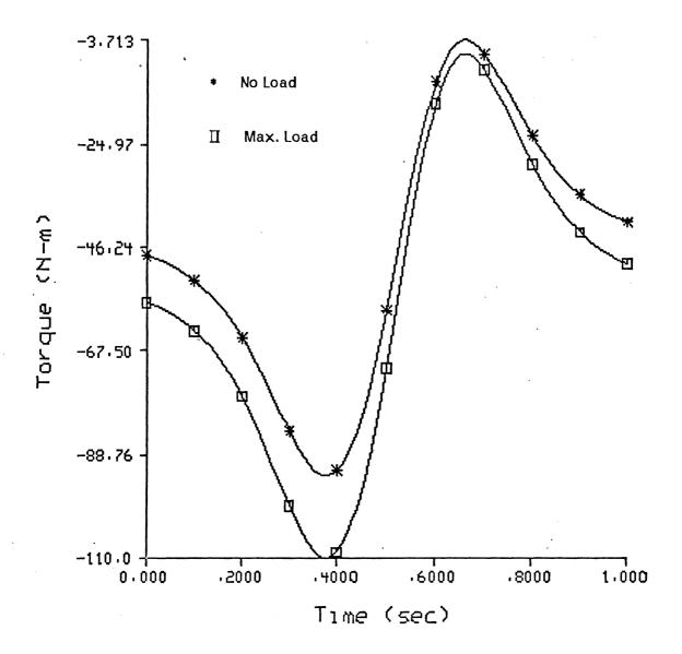
Figure 13 Variation of the Applied Torque ( Joint 2 )
