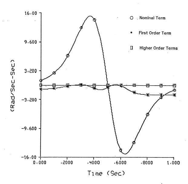
Figure 5 Contributions of the First Order Term and the Higher Order Terms in the Linearization of the Dynamic Model ( Joint 3 )
