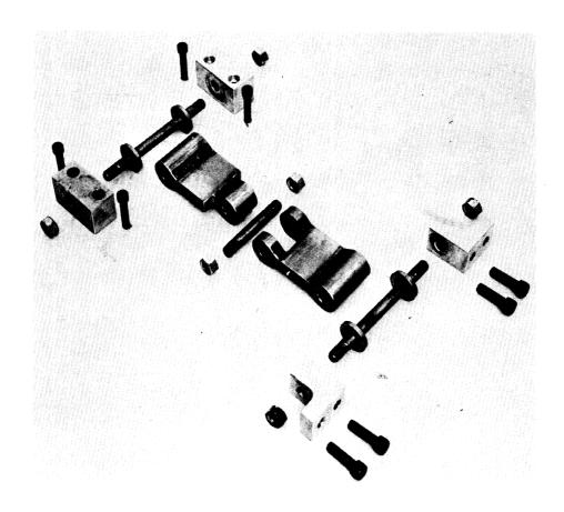
The next sub-assembly is used for control of sway of the device during its axial plunging.
