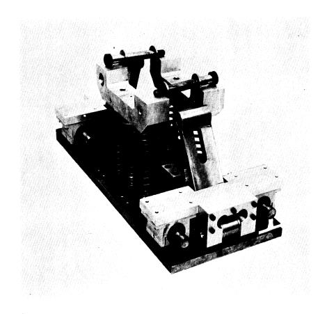
Unlock the set screw of the friction block and slide platform until bushing of pivoting arm is lined up with the cradle holes.
