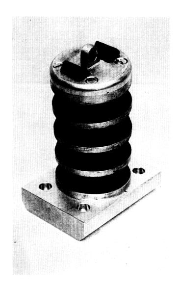
Attach the neck adaptor to the top of the neck as shown. Use 4 flat head screws [HITS-002-20].
