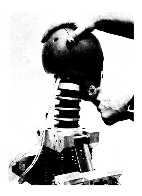
The Helmet Impact Test System (HITS) is designed to test the performance of industrial helmets. In order to operate the device, you need a mechanism for dropping a weight (drop tower), a test floor/platform to which the device base will be bolted, and signal conditioning and recording equipment for a minimum of six data channels.
