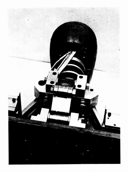
Attach the two upper pivots of the sway control assembly to the cradle face using 4 screws [HITS-002-3 ].
