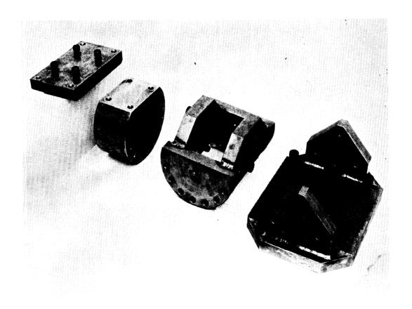
The massive mounting base consists of a welded base assembly (HITS-220] with two uprights, a welded cradle assembly [HITS-210] with two semi-circular sides, a rotating cylinder [HITS-202] with a flattened top, and an upper platform [HITS-201].
