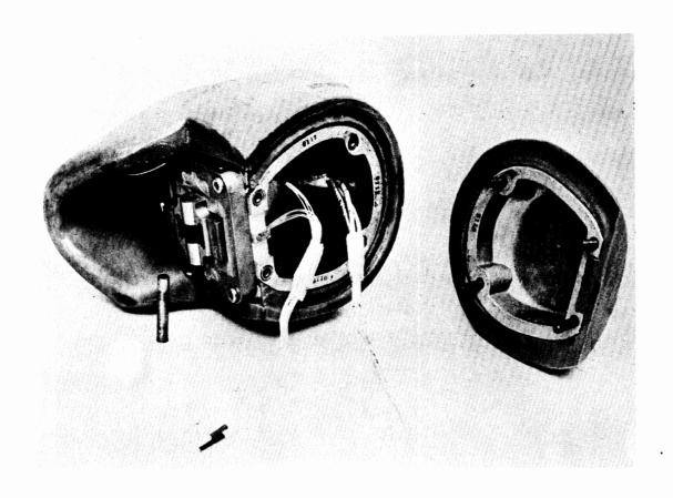
Using drafting tape, arrange cables inside the head and tape the 3 accelerometer cables into one bunch and the two load cell cables into another bunch. Place the 2 bunched cables into the two slots in the back of the head.
