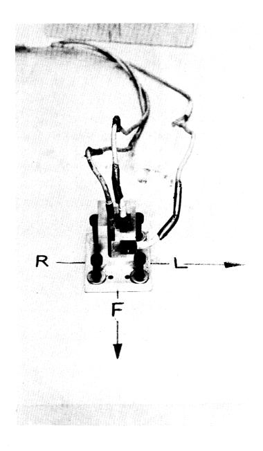
Install 3 Endevco uniaxial accelerometers [model 2264] on triax [HITS-011] using #0-80 screws.
