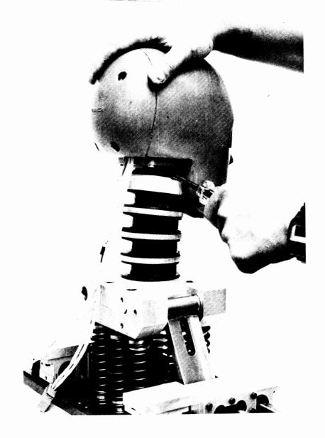
Finally, place the head assembly on the neck assembly by slipping the yoke of the neck load cell over the bushing of the neck adaptor plate.
