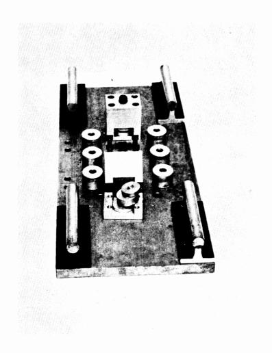
Install 4 guide rod assemblies [HITS-153] at the corners of the thorax lower plate [HITS-161] using 16 screws [HITS-002-13].
