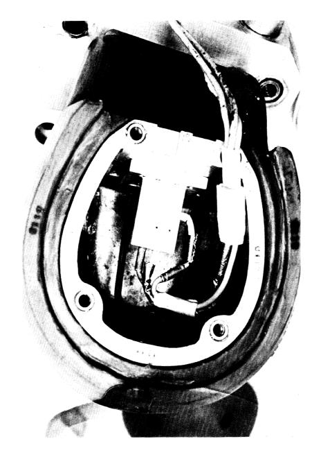
Use 4 screws [HITS-002-70] and washers attach the triaxial accelerometer package inside the dummy head.
