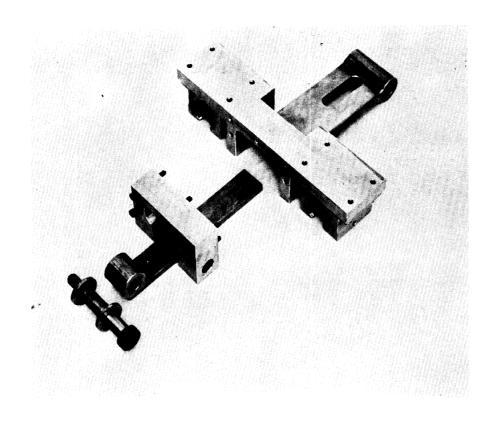
Using 1 shoulder bolt [HITS-002-30] and 2 brass spacers [HITS-003], attach the friction bar [HITS-142] to the friction bar pivot [HITS-141].
