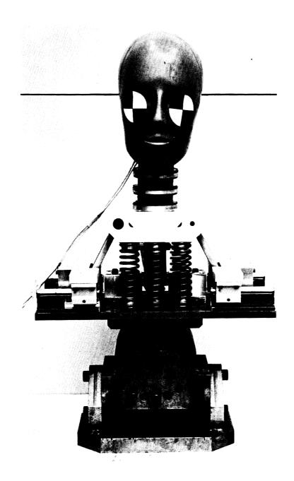
The Helmet Impact Test System (HITS) consists of three major sub-assemblies: the head/neck including transducers for 6 data/channels, the thorax which provides axial plunging motion for the head, and the mounting base which allows control of location and direction of impact.
