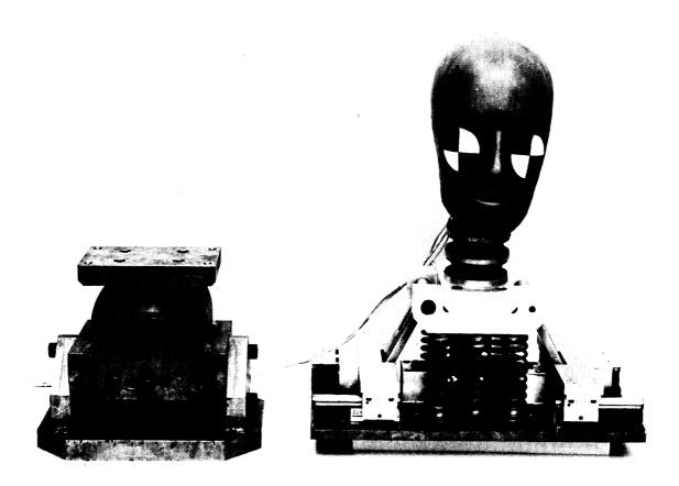
When the mounting base is properly bolted to the laboratory test fixture using 4 bolts [HITS-002-1] and the drop tower (or similar device) is aligned with the device, the head/neck/thorax assembly (shown on the right) may be attached to the fixed mounting base using 4 screws (HITS-002-9].
