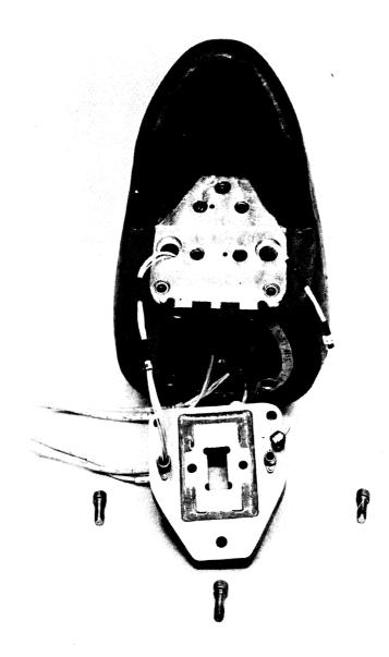
Through the two holes at the head base, pass the two 7-pin miniconnectors and cables from the inside toward the outside.
