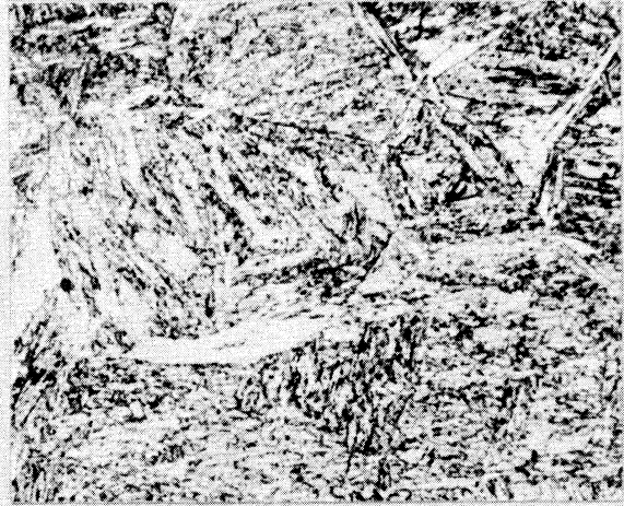
(a) Air Cooled from 1850°F + Oil Quenched from 1750°F (0.8-Inch Round). Avg. BHN - 506
