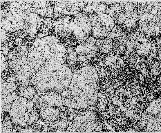
(b) Air Cooled from 2200°F + Tempered 7 Hours at 1250°F. Avg. BHN - 362
