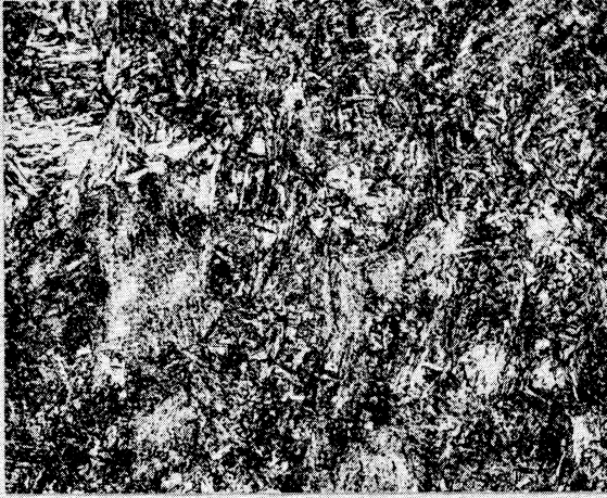
(a) Hot Rolled 25 Percent in Three Passes during Air Cooling from 2100°F to 1800°F. Avg. BHN - 386
