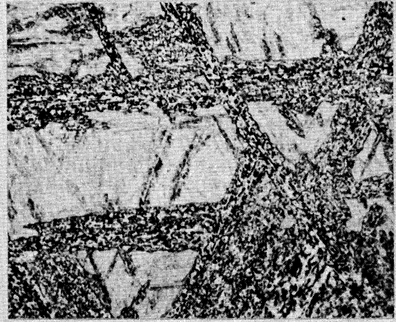
(a) Air Cooled from 2100°F to 1800°F and then Hot Rolled 25 Percent in One Pass. Avg. BHN - 366
