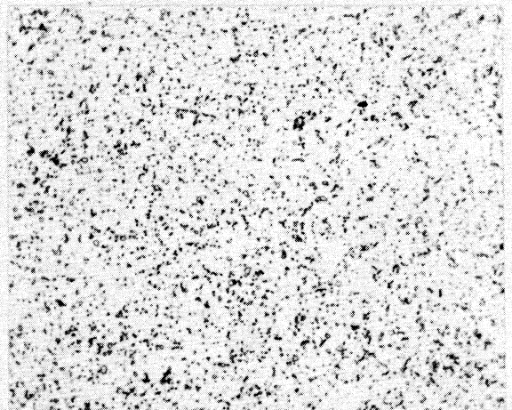
(c) Same As in (b) + Creep Tested 763 Hours at 1100°F and 19,000 psi. BHN - 276
