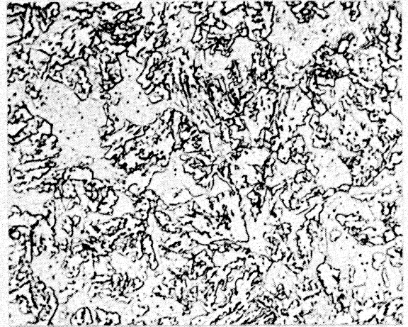
(a) Austenitized at 1850°F and Isothermally Transformed 2 Hours at 850°F to Upper Bainite (0.4-Inch Round). Avg. BHN - 447
