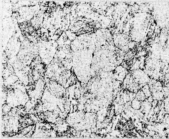
(b) Same As in (a) + Tempered 2.5 Hours at 1250°F. Avg. BHN - 358
