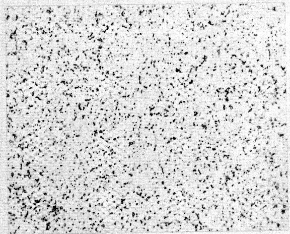
(c) Same As in (b) + Creep Tested 1032 Hours at 1100°F and 19,000 psi. BHN - 267
