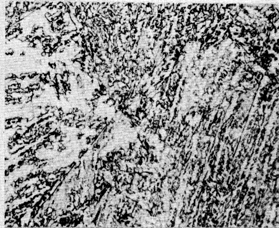
(a) Air Cooled from 2200°F to 1900°F and then Hot Rolled 25 Percent in One Pass. Avg. BHN - 381
