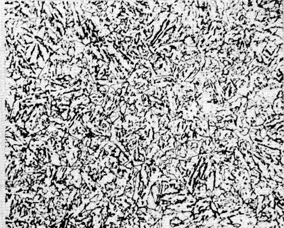
(a) Austenitized at 1850°F and Isothermally Transformed 0.3 Hours at 750°F to Middle Bainite (0.4-Inch Round). Avg. BHN - 364
