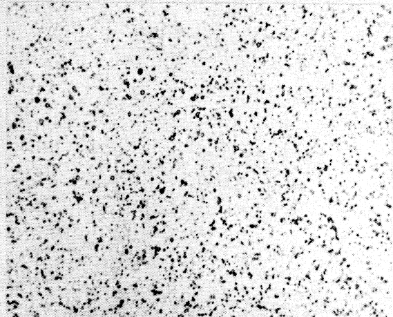
(c) Same As in (b) + Creep Tested 995 Hours at 1100°F and 19,000 psi. BHN - 259
