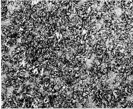
(a) Isothermally Transformed Stepwise at 900° and 700°F to 50 Percent Upper Bainite + 50 Percent Lower Bainite. Avg. BHN - 353
