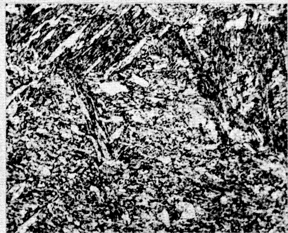
(b) Same As in (a) + Tempered 1.75 Hours at 1200°F. Avg. BHN - 307
