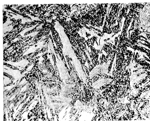
(b) Air Cooled from 1850°F + Air Cooled from 1750°F (0.8-inch Round). Average BHN - 408
