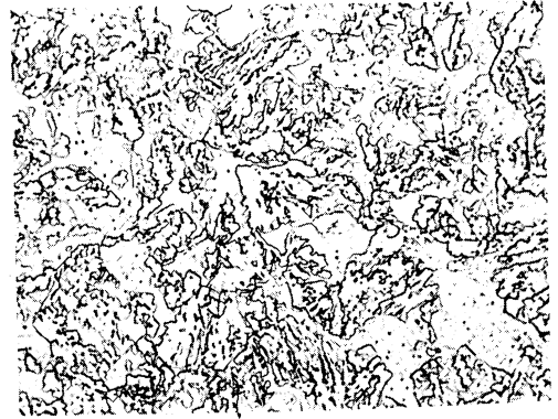
(a) Isothermally Transformed to Upper Bainite (0.4-inch Round). Average BHN - 447
