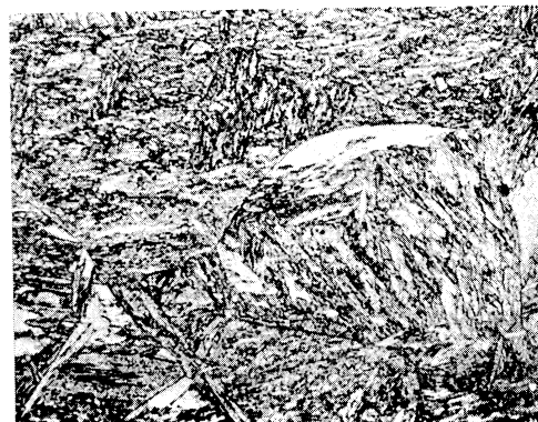
(a) Air Cooled from 1850°F + Oil Quenched from 1750°F (0.8-inch Round). Average BHN - 506
