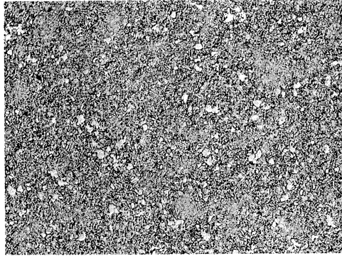
(a) Air Cooled from 1850°F in Firebrick Jacket to Simulate Cooling Cycle at Center of a 3-inch Round. Average BHN - 365
