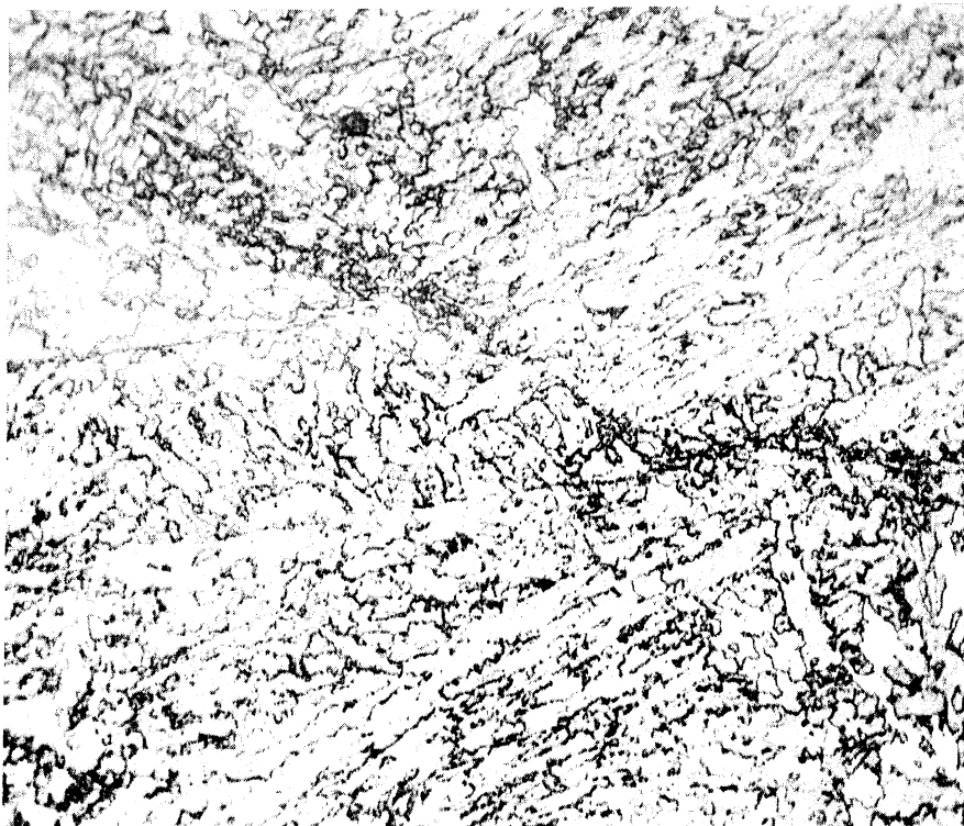
Figure 8. - "17-22-A" V steel heated 1 hour at 2200°F., air cooled to 1900°F., rolled 50 percent reduction in 2 passes, and air cooled to room temperature + tempered 6 hours at 1250°F. No recrystallization during rolling.
