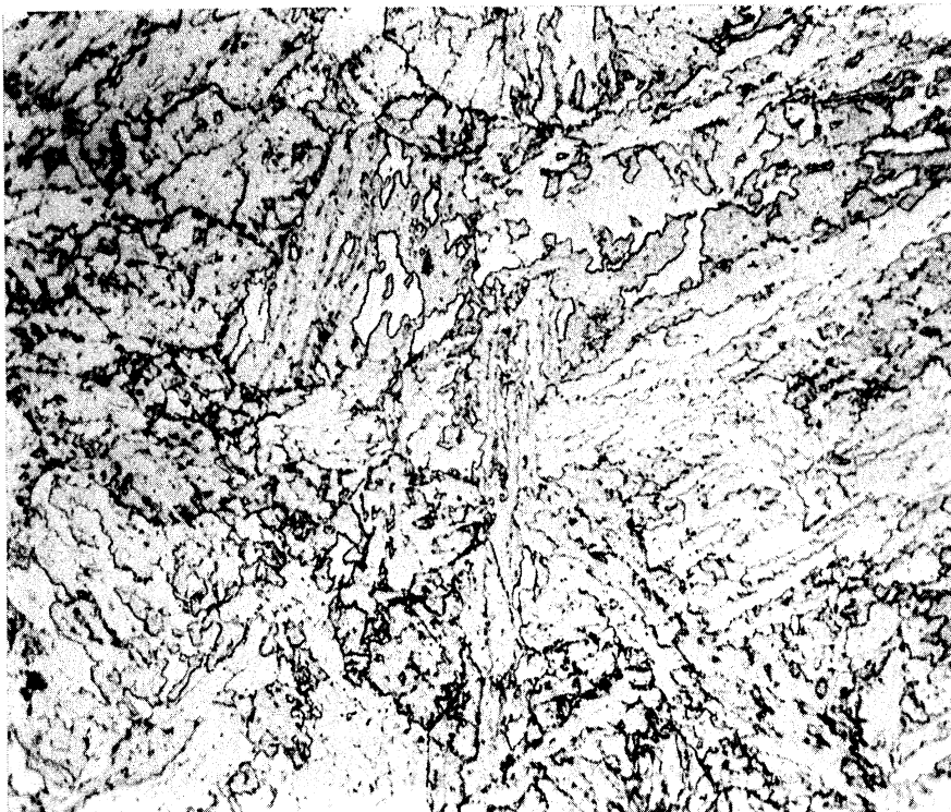
Figure 7. - "17-22-A" V steel heated 1 hour at 2200°F., air cooled to 2000°F., rolled 50 percent reduction in 2 passes, and air cooled to room temperature + tempered 6 hours at 1250°F. Partial recrystallization during rolling.
