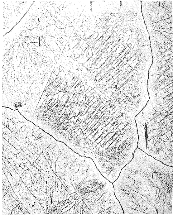
(b) Strained in Tension to 4% Elongation at 1600°F at a Constant Strain Rate of 100%/hr.
