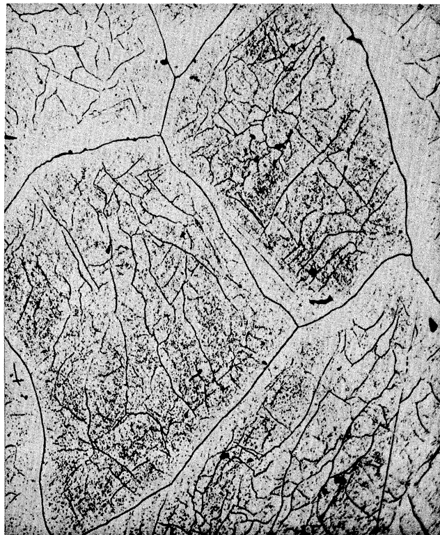
(c) 3.5% Creep Strain in 20 Hours at 1500°F and 3,325 psi. X250.
