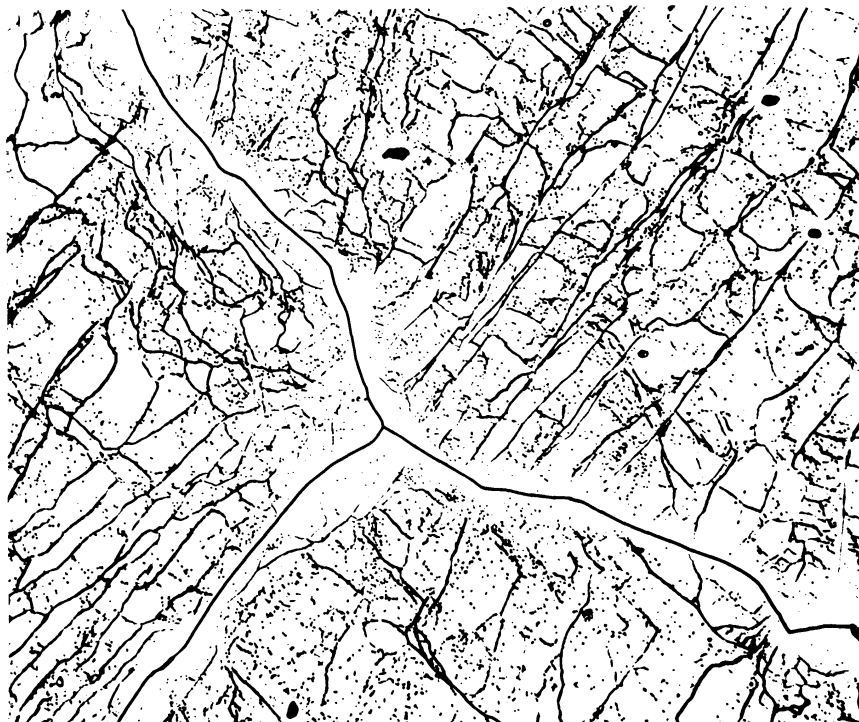
(c) 2.69 Percent Elongation; Decelerating Creep. Mag. 500X.
