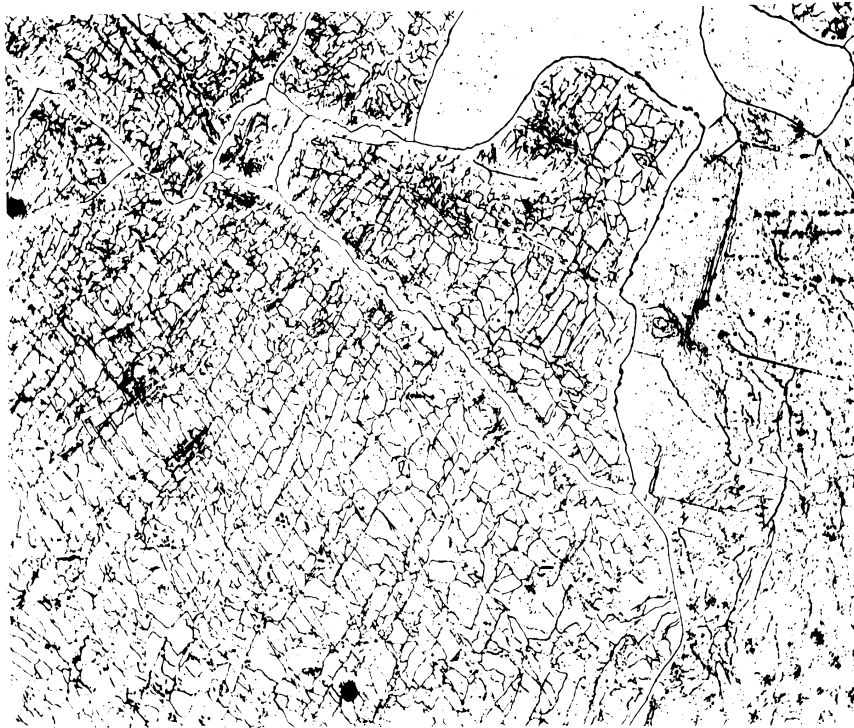
(e) 5.18 Percent Elongation; Accelerating Creep. Mag. 100X.
