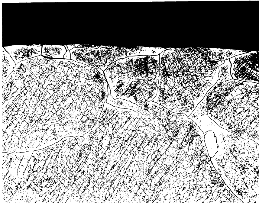
(b) Photomicrograph of the Edge of a Specimen Creep Tested In Vacuo at 1550°F. Mag. 100X.
