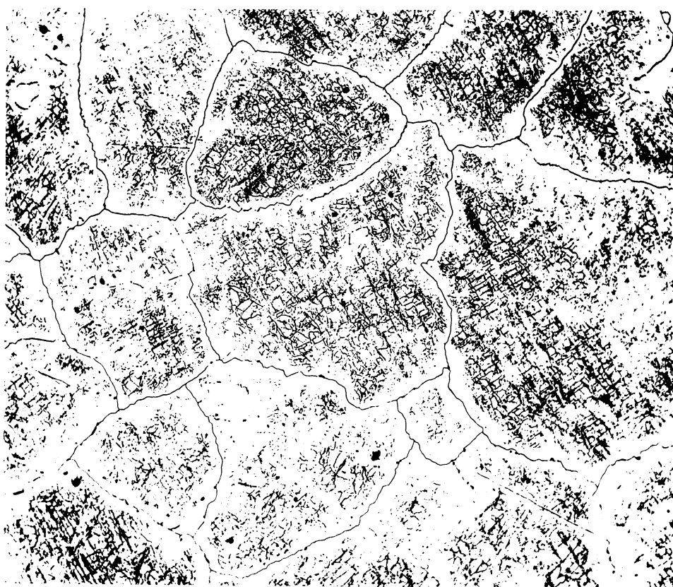
(b) Creep Tested at 1400°F and 4,790 psi to 6.60 Percent Elongation in 6.6 Hours. Mag. 100X.
