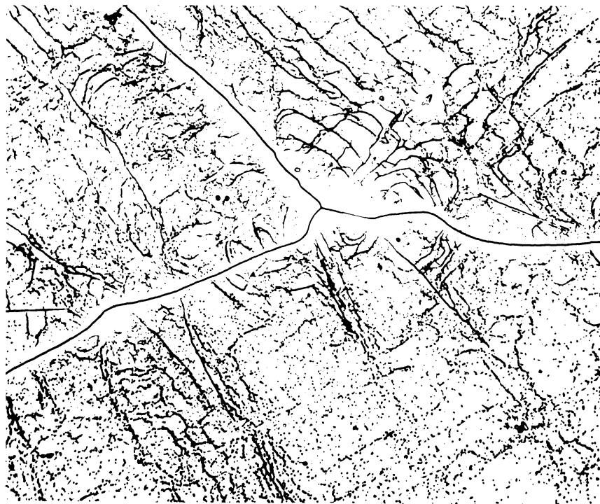
(b) 2.04 Percent Elongation; Decelerating Creep. Mag. 500X.
