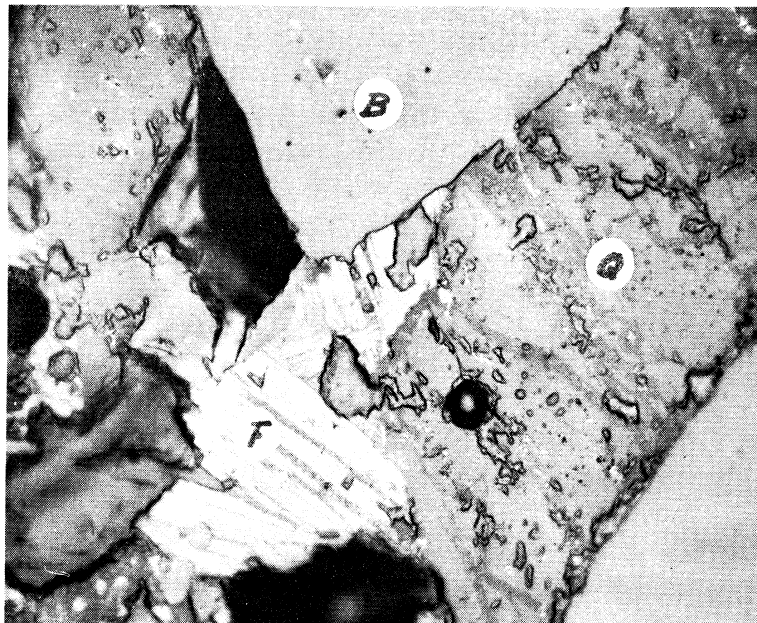
Iron-0.23% manganese alloy Magnification: 500X
