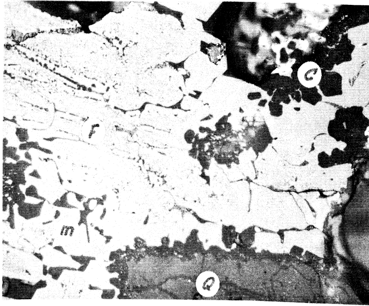
Iron-8.60% manganese alloy Magnification: 500X
