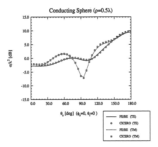
Figure 4.5: TM and TE bistatic scattering pattern from a perfectly conducting sphere of radius  $\frac{\lambda}{2}$  for axial incidence.
