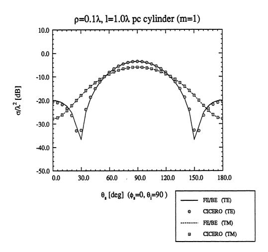
Figure 4.2: Mode 1 TM and TE bistatic scattering pattern from a perfectly conducting circular cylinder of length  $1\lambda$  and radius  $0.1\lambda$  for broadside incidence.
