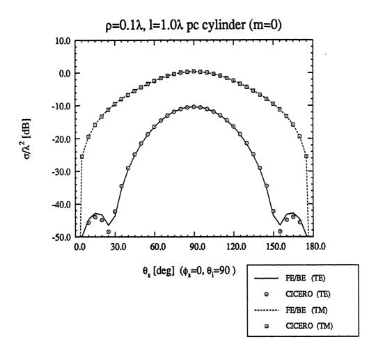
Figure 4.1: Mode 0 TM and TE bistatic scattering pattern from a perfectly conducting circular cylinder of length  $1\lambda$  and radius  $0.1\lambda$  for broadside incidence.
