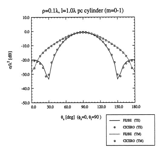
Figure 4.3: Modes 0+1 TM and TE bistatic scattering pattern from a perfectly conducting circular cylinder of length  $1\lambda$  and radius  $0.1\lambda$  for broadside incidence.
