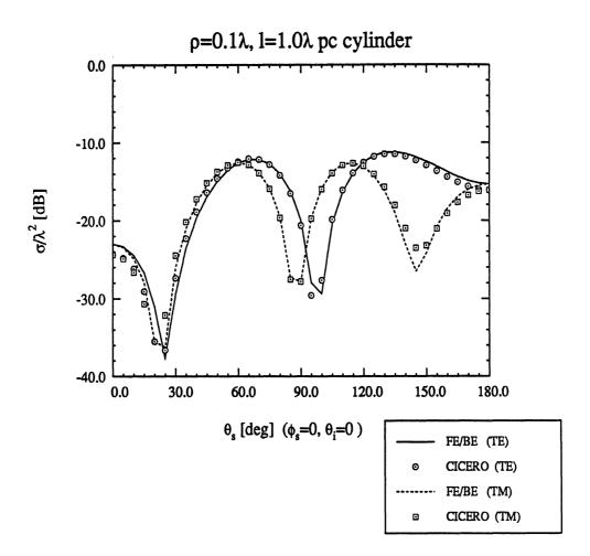
Figure 4.4: TM and TE bistatic scattering pattern from a perfectly conducting circular cylinder of length  $1\lambda$  and radius  $0.1\lambda$  for axial incidence.
