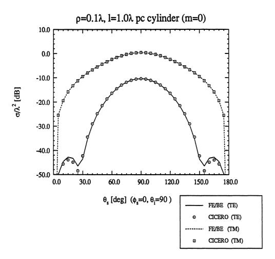
Figure 4.1: Mode 0 TM and TE bistatic scattering pattern from a perfectly conducting ircular cylinder of length  $1\lambda$  and radius  $0.1\lambda$  for broadside incidence.
