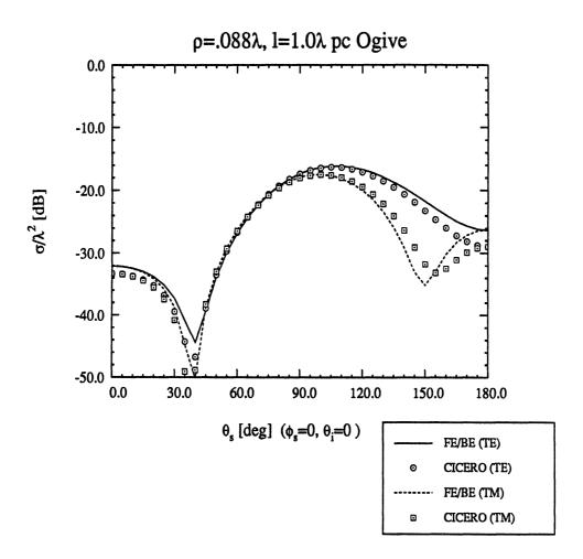
Figure 4.6: TM and TE bistatic scattering pattern from a perfectly conducting ogive length  $1\lambda$  and maximum radius of  $0.088\lambda$  for axial incidence.
