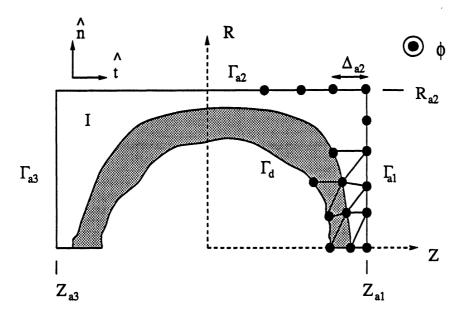
Figure 2.2: Cross section of a generating surface enclosed by the fictitious boundary  $\Gamma_a$ .
