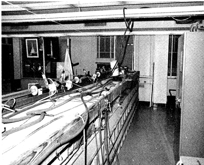
Fig. 16. - Laser amplifier and optical bench.
