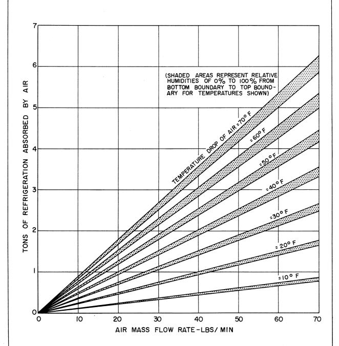
Fig. 1. Refrigeration absorption by air as a function of mass flowrate, temperature drop, and relative humidity.
