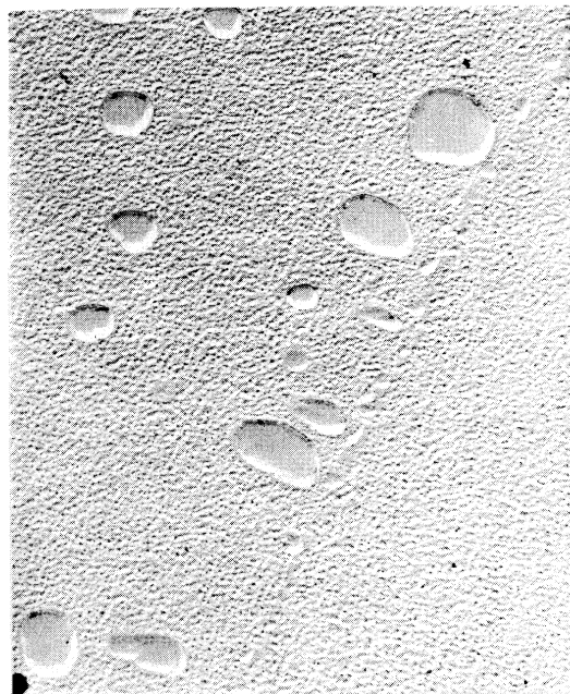
b. As rolled + 4 hours at 1975°F, air cooled; light micrograph.
