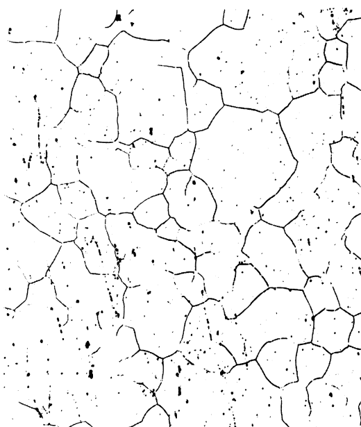
X100D Homogenized 1 hour before rolling plus 1 hour during rolling
