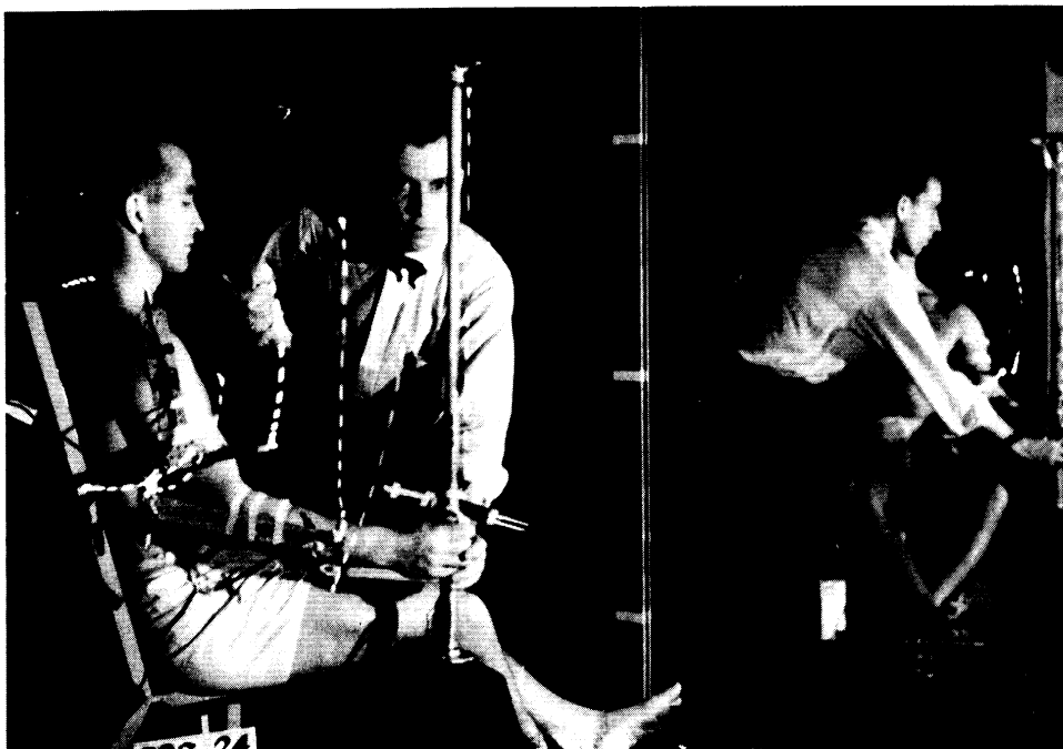
Fig. 7. This figure, showing the path of flashes of neon lights attached to the hand, forearm, and arm, is comparable to Fig. 4 for the lower limb. As the subject's hand is moved up or down relative to the vertical pipe, the angular relations of the passive limb segments change at each joint. The pattern of segment movement as indicated by light paths provides data for analysis of axes and distances between axes.
