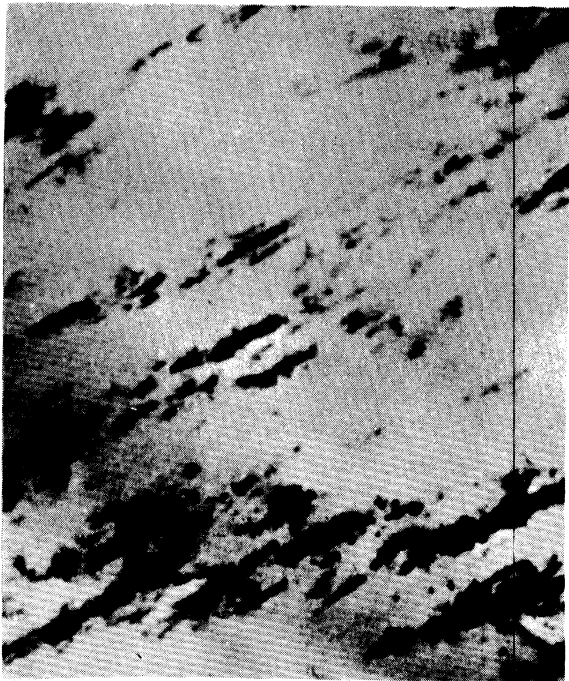
Figure 29. Defect Present in the Specimen Failed at Medium Strain. 15,000X
