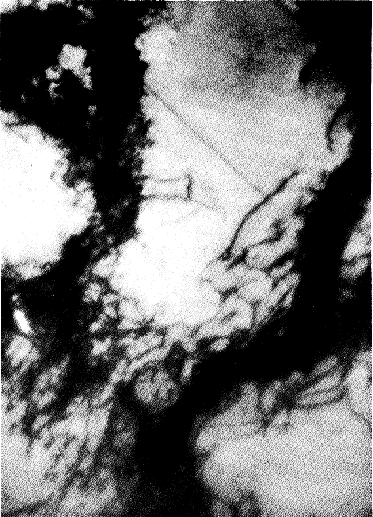
Figure 35. Cellular Structure of Dislocation Tangles Formed at High Strain. Numerous dislocation loops and individual tangles can be seen. 200,000X
