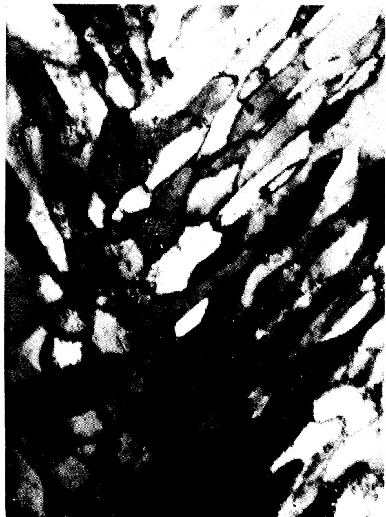
Figure 46. Subgrains Found in the Failure Specimens Fatigued at High Strain. 10,000X
