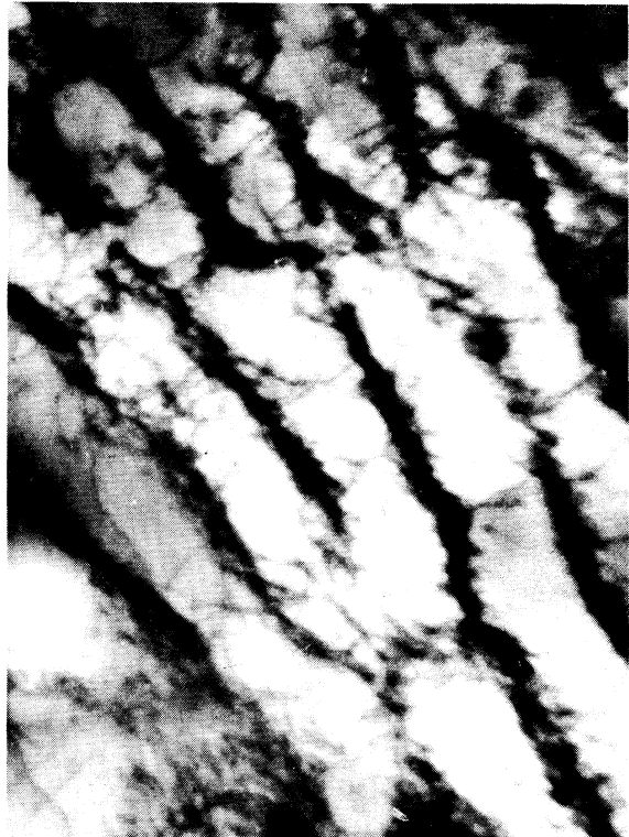
Figure 44. Rows of Dense Tangles Resulting from High Strain Reversed Cycling. 30,000X
