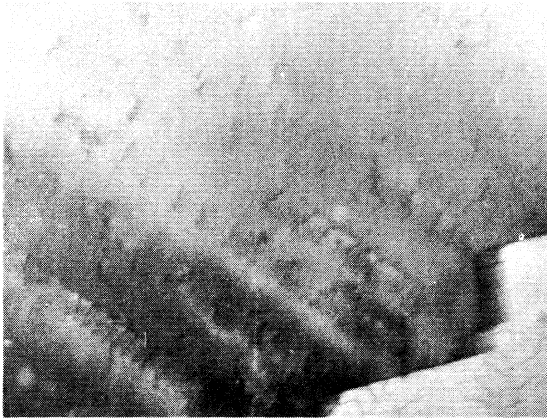
Figure 11. Transmission Micrograph Showing Dislocation Pile-ups Resulting from a Unidirectional Tensile Strain of 0.3 Percent. 8,000X
