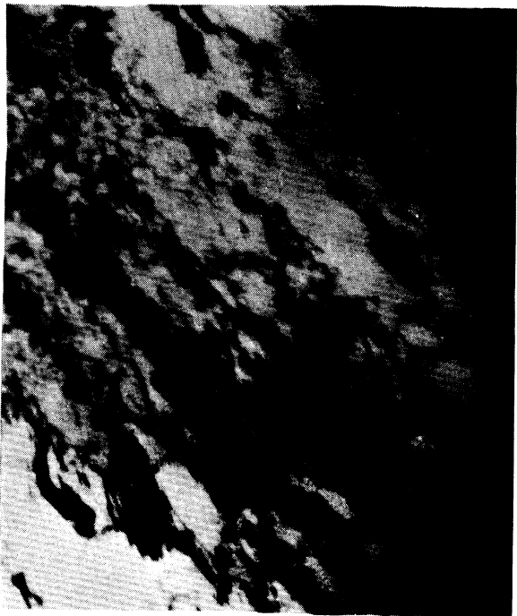
Figure 30. Typical Bands of Extremely Dense Defect Structure in the Specimen That Was Failed at Medium Strain. 15,000X
