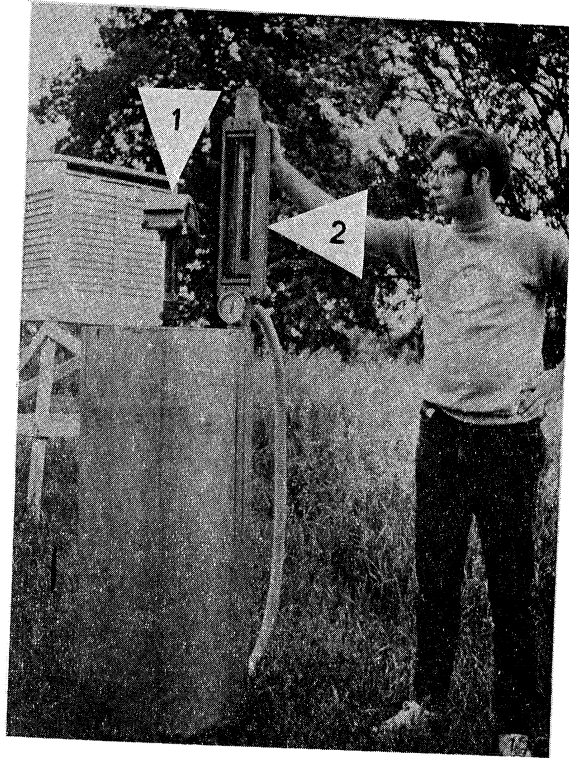
Figure 2. Hi-volume air sampler, supplied by Argonne National Laboratory for use at the base station. Indicated in the photograph are the (1) intake and (2) flow rate meter.
