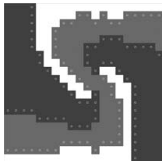
Fig. 6 Boundary elements are detected on the quarter part of the square symmetric structure
