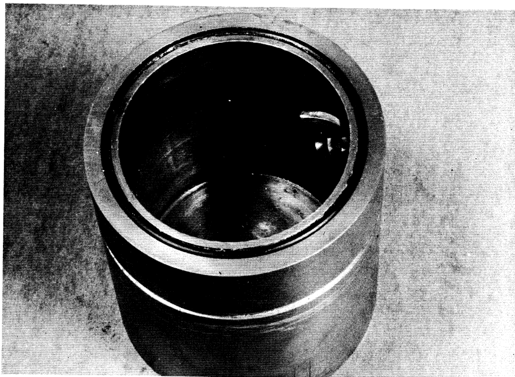
Figure 10B. The cathode after cleaning with soap and water.
