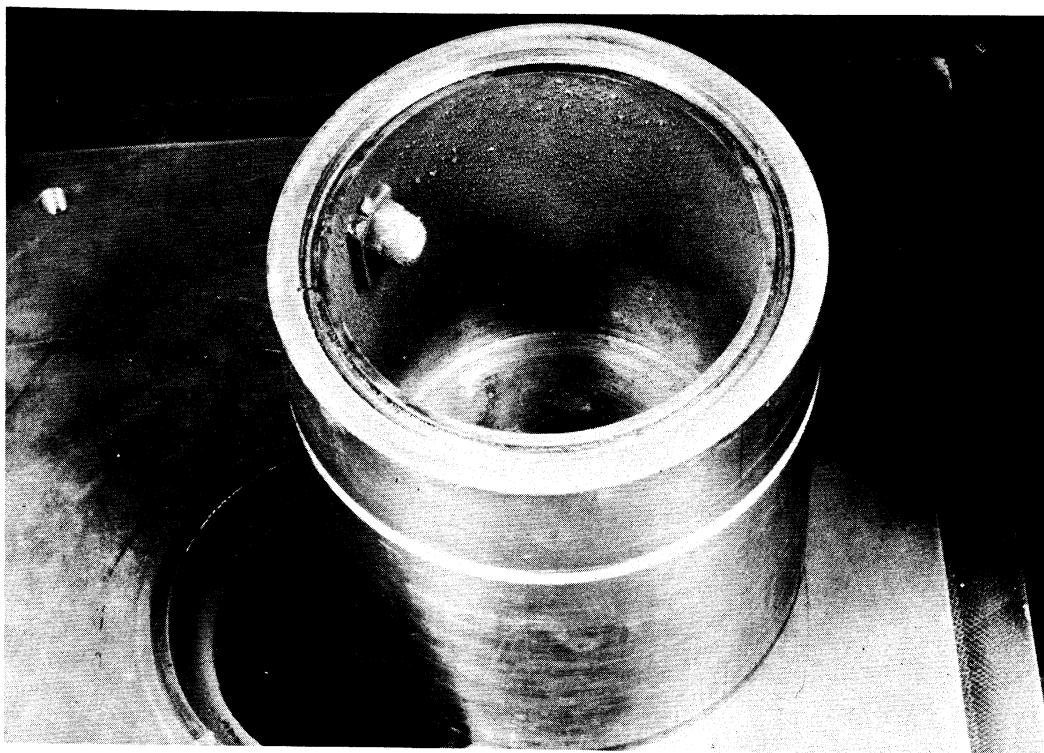
Figure 10A. The anode, the upper half of the chamber, after the first experiment at 30,000 amperes and 54,000 joules.
