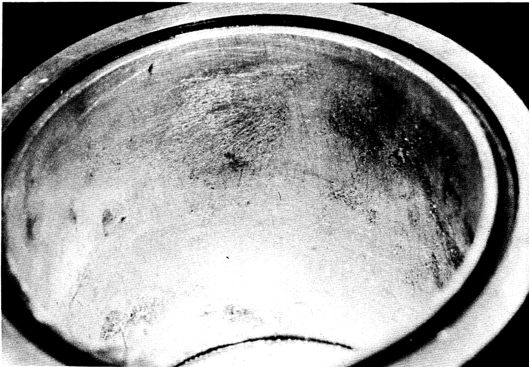
Figure 12B. The anode marks.
