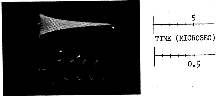
Fig. 14. Oscillogram of current in discharge circuit when corona electrodes are shorted.
