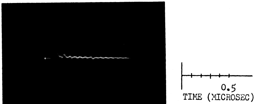
Fig. 10. Oscillogram of pulse voltage across corona electrodes with minimum circuit inductance.
