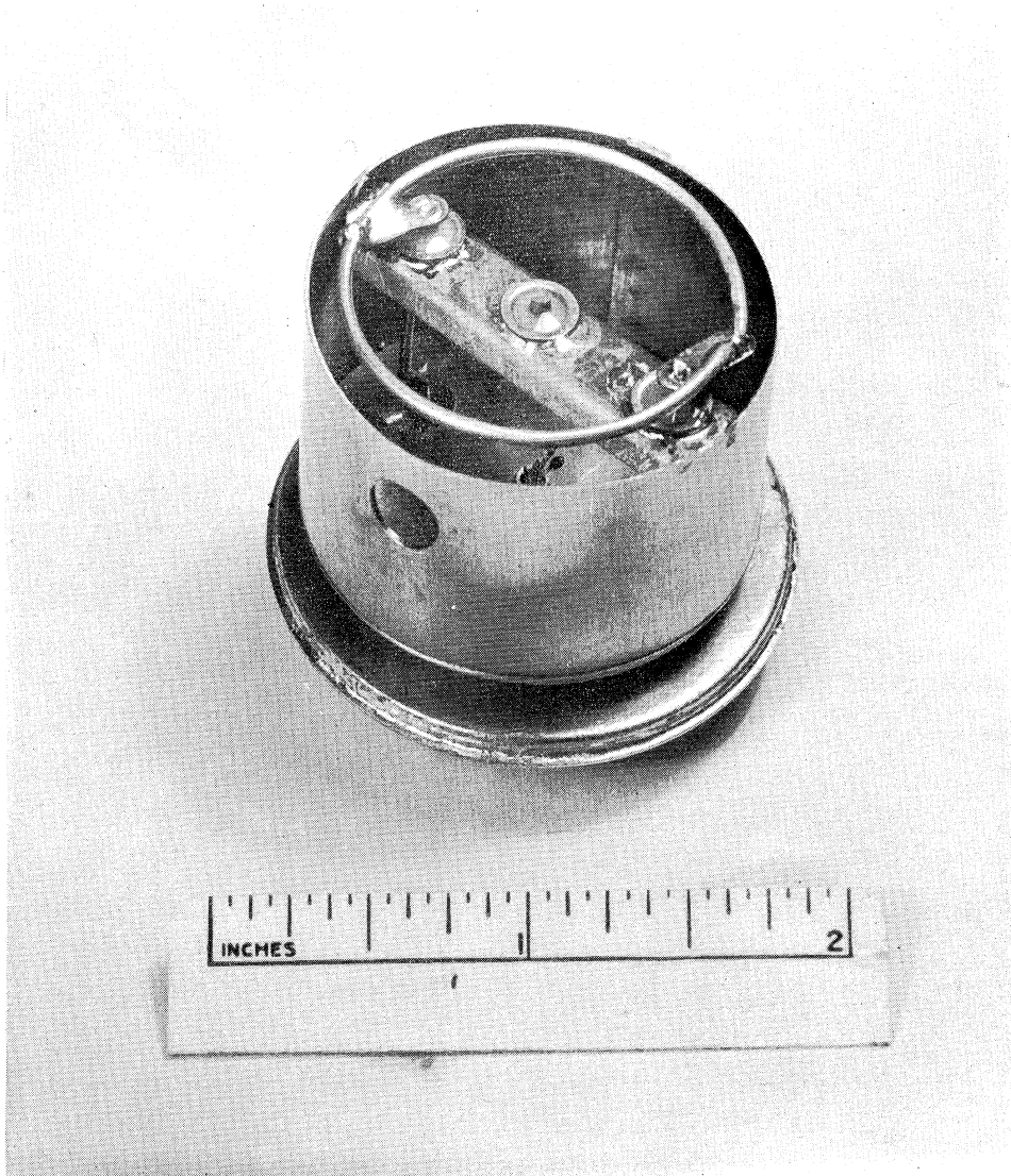
Fig. 4.29. Ionization-chamber element assembly.
