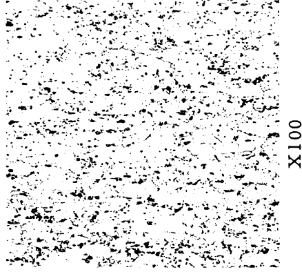
Rolled 25 percent at 2000°F plus 15 percent at 1600°F
