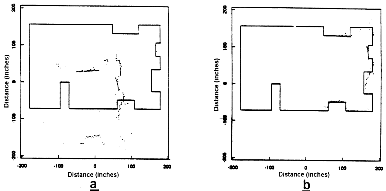
Figure 8.5: Map and range data (a) before registration and (b) after registration. (Reproduced and adapted from [Cox, 1991]).
