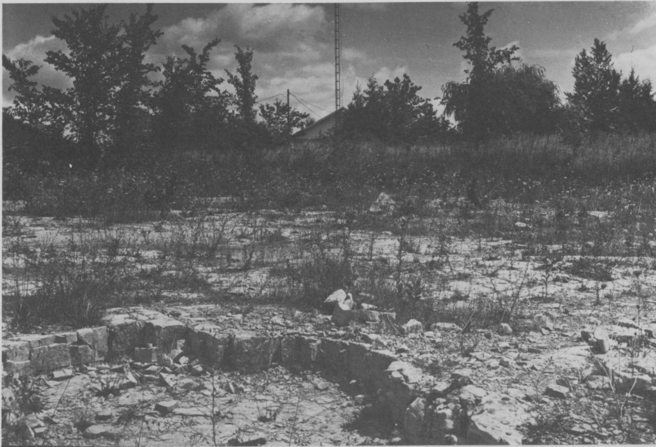
TEXT-FIG. 25 -- Koehler Limestone exposed in the quarries of the Onaway Stone Company near Onaway. The jointing is used to advantage in the hand-quarrying of particular layers, which are then scored with diamond saw and broken into brick-size blocks for building facings and trim. Locality 34-2E-5 N. Photograph by Kesling, 1969.
