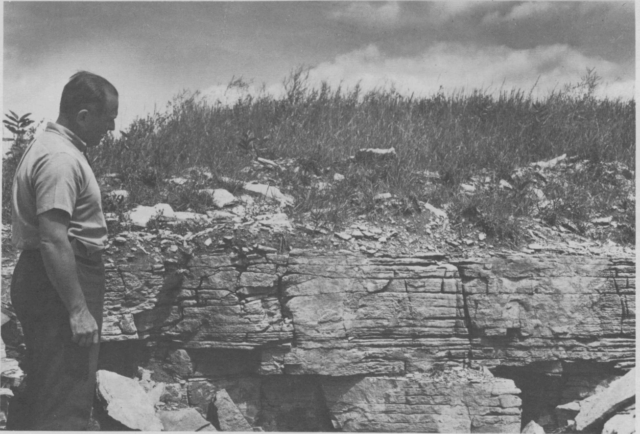
TEXT-FIG. 28 -- Koehler Limestone exposed in Onaway Stone Company Quarry. Locality 34-2E-5 N. Weathered surface developed along a joint exposes the irregular bedding. Quarrymen avoid the beds of irregular thickness, as well as those which fail to break readily when scored by diamond saw; as a result, the quarry area is congested with discarded pieces of limestone stacked at temporarily convenient areas. Photograph by Kesling, 1969.
