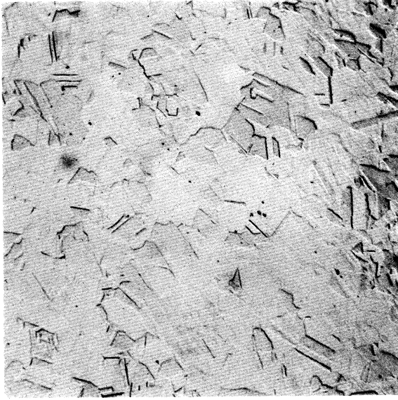
Fig. 10. 500x, dichromate etch. This photomicrograph shows little oxide and grain boundaries.
